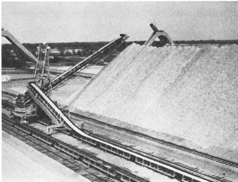
WOOD CHIPS are the form in which chemical pulping is done. Debarked logs are put into a chipper, which reduces them to the material seen here being moved from chipper to storage pile.
