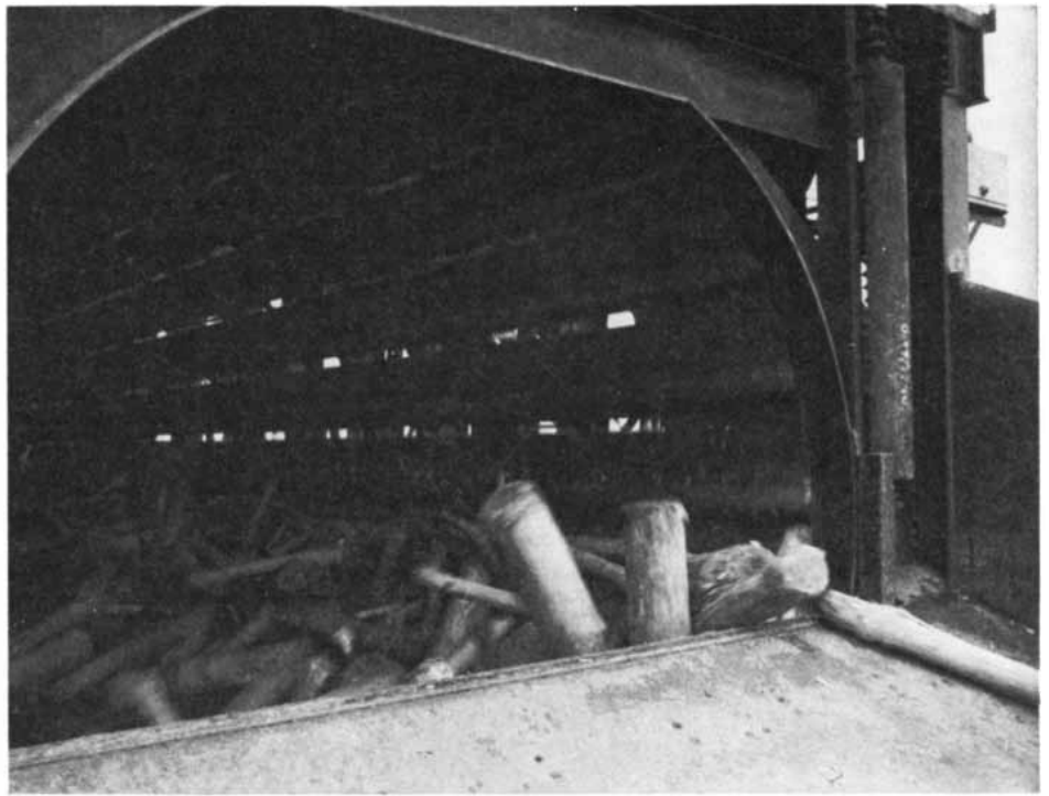
DEBARKING DRUM removes the bark from logs by revolving and causing them to strike one another repeatedly. The bark, which is a waste product in pulping, falls between openings of drum.
