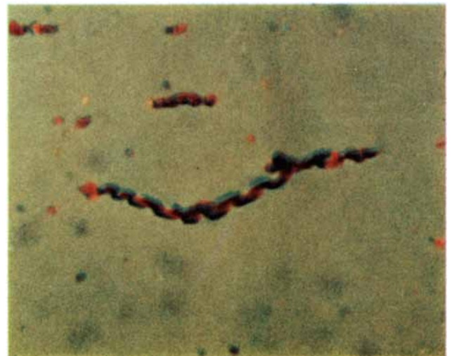
SPIRAL CUTTING-WEAR PARTICLE , very similar to chips produced by a metal-cutting lathe, is shown enlarged 1,600 diameters.
