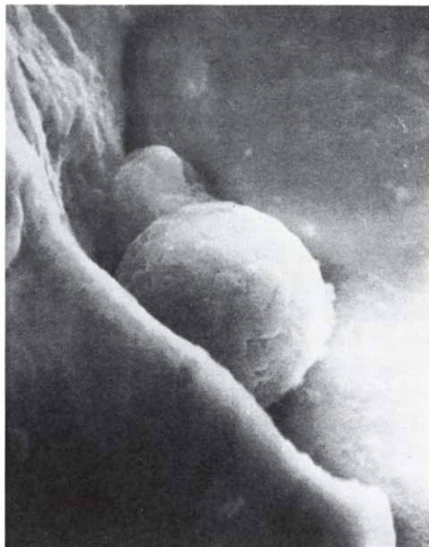
SPHERE IN CRACK appears to be in the process of formation. The surface of the sphere is covered with laminae that have not yet been smoothed out. Magnification is about 6,000 diameters.
