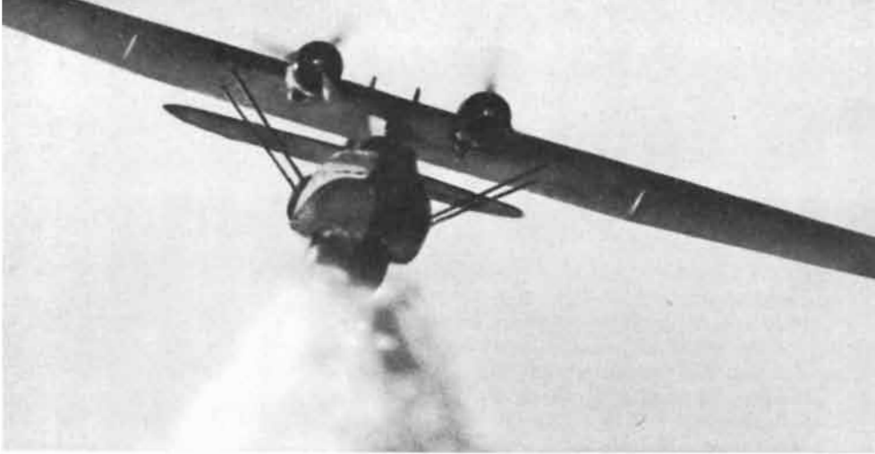
CANSO SPREADS 800 GALLONS OF WATER AT A TIME, SCOOPED FROM NEARBY LAKES IN HIGH-SPEED TAXI RUNS.
