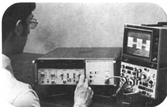
The new HP 5345A counter with optional frequency converter plug-in automatically measures CW or very brief pulsed signals well into the microwave region. Here, the counter measures the pulsed signal displayed on the scope.
