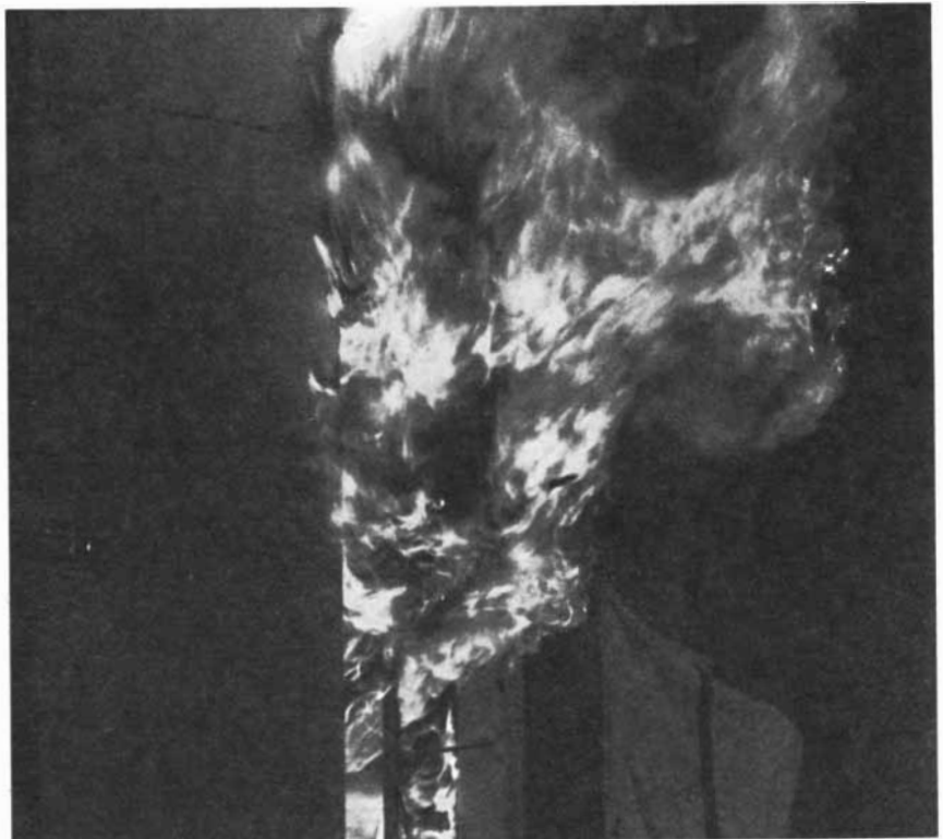
FLASHOVER IN BEDROOM started 17 minutes and 35 seconds after ignition. The delay in flashover, which would have given occupants more time to escape and firemen more time to respond, was thought to be due in part to the fact that the plastic-fiber drapes melted and fell to the floor in six minutes. Retardants in drapes might similarly delay flashover.
