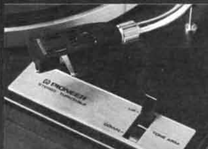
Gentle viscous damped cueing control.
