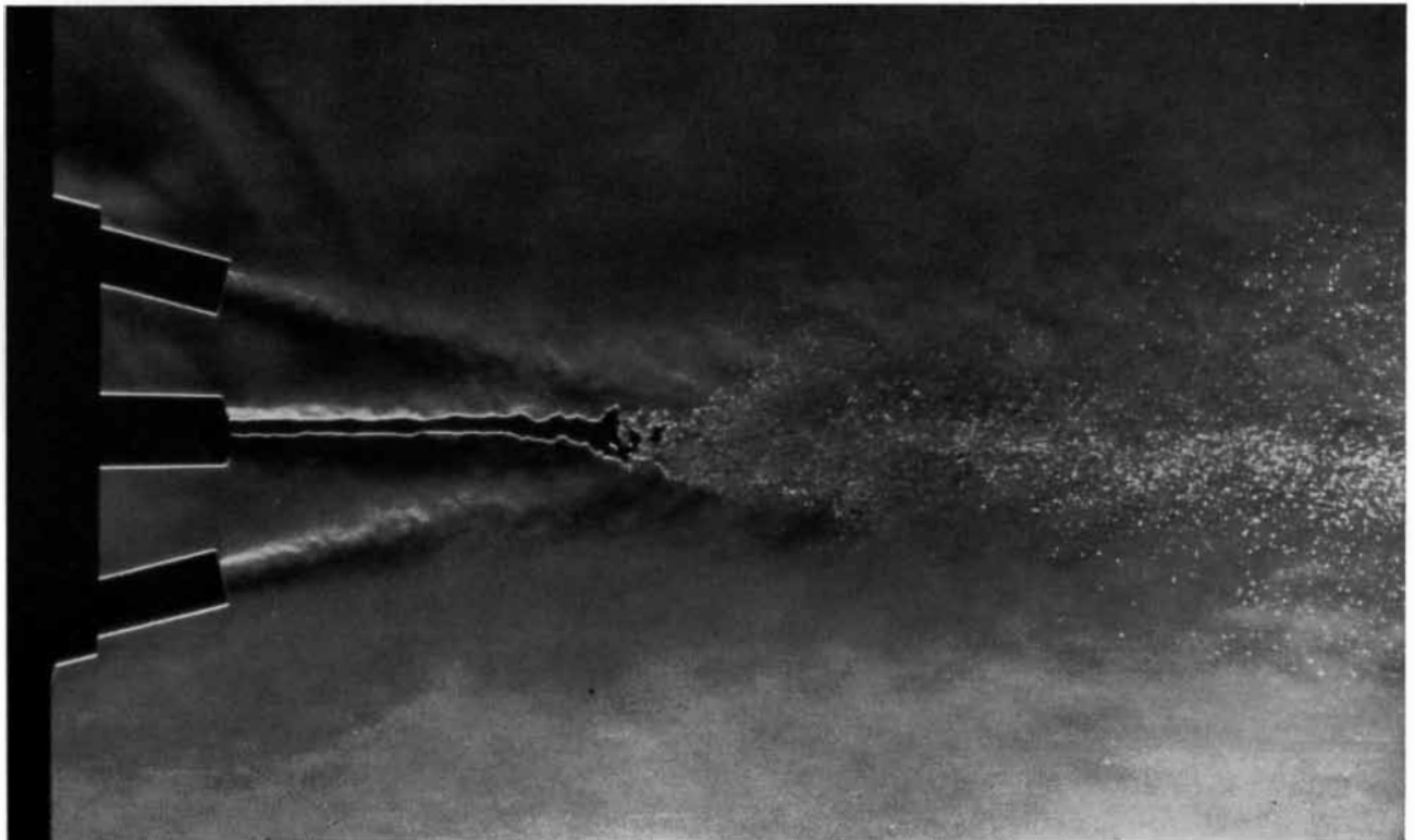
Atomization of liquid in jets of nitrogen
