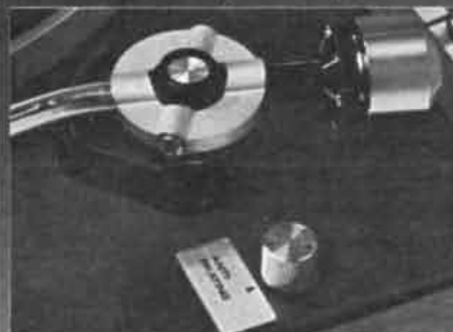
Anti-skating control insures perfect tracking.
