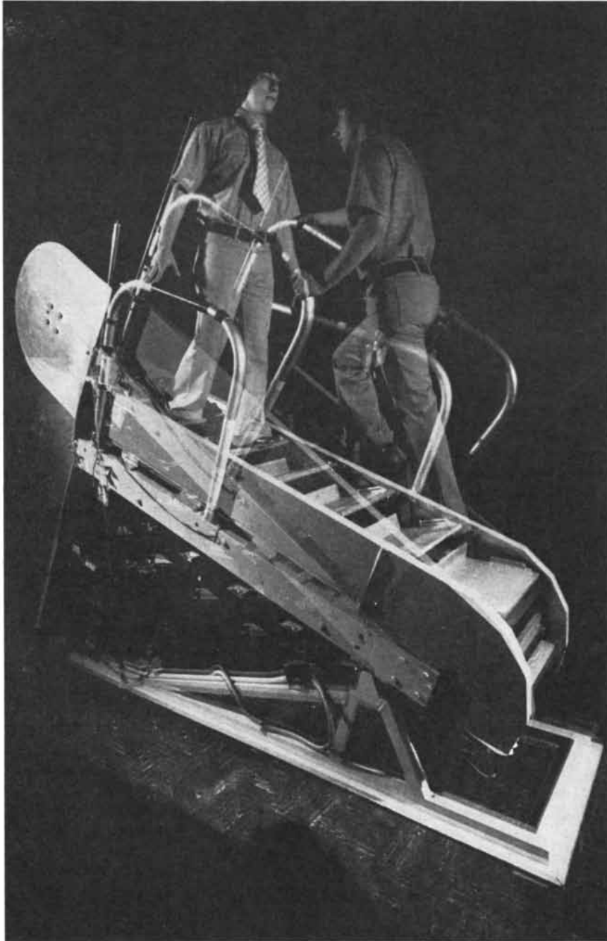
MECHANICAL STAIRWAY enabled the experimenters to test a number of different riser and tread combinations, pitches and speeds of ambulation for both their effect on the human gait and the amount of energy required to climb under various conditions. Here the machine appears in a double exposure that portrays how it can be set at different angles of pitch and how it serves for both ascent and descent. The apparatus is at the Helen Hayes Hospital in West Haverstraw, N.Y., a state facility where the experimental work was done.
