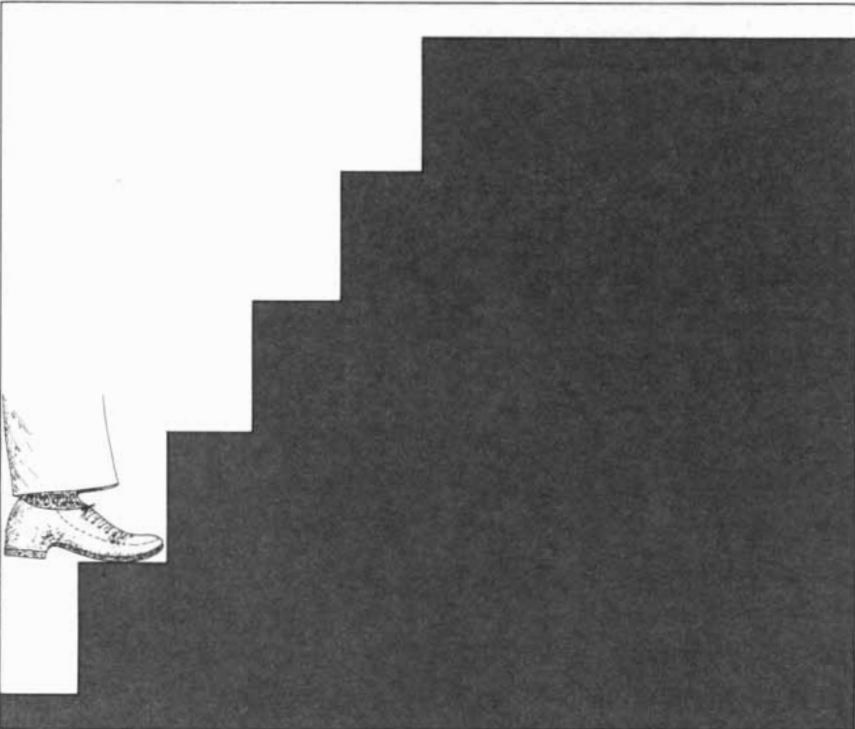
RISER AND TREAD COMBINATIONS are portrayed according to a formula derived some 300 years ago by François Blondel, director of the Royal Academy of Architecture in Paris. He held that the depth of the tread should be 24 inches minus two times the height of riser. Application of formula is shown here for risers of five ( top ), seven and nine inches.
