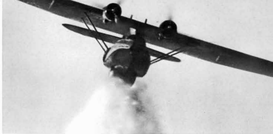
CANSO SPREADS 800 GALLONS OF WATER AT A TIME, SCOOPED FROM NEARBY LAKES IN HIGH-SPEED TAXI RUNS.
