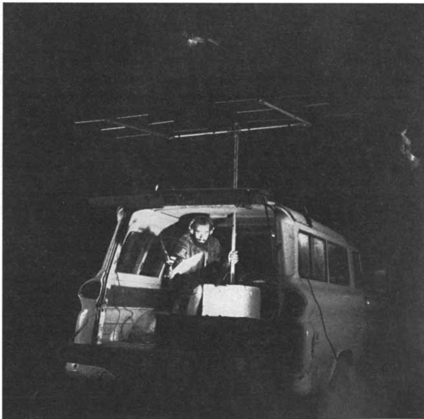
NIGHT NAVIGATION of pigeons is being studied by Cornell workers. Pigeons with radio transmitters on their back are released and tracked by a radio receiver in the truck. In this time exposure three successive light flashes were used to illuminate the flying pigeon.
