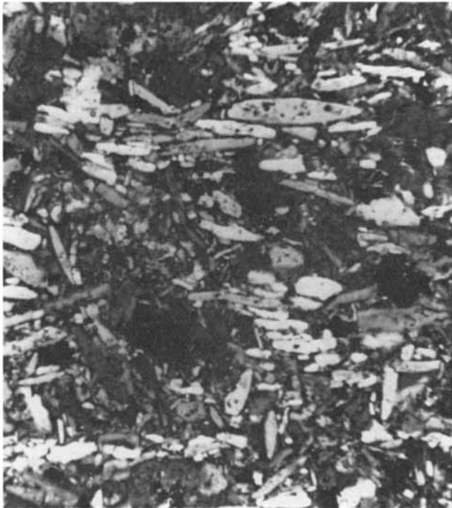
MATRIX OF A C3 CHONDRITE , the Allende meteorite, is viewed in photomicrograph made by R. H. Beauchamp of Battelle Pacific Northwest Laboratories. Platelike material is half forsterite ( Mg_2SiO_4 ) and half Fe_2SiO_4 . Dark opaque grains are troilite ( FeS ). Composition is similar to composition predicted for materials that reached equilibrium with solar nebula between 700 and 400 degrees. The width of the field of view is 108 micrometers.
