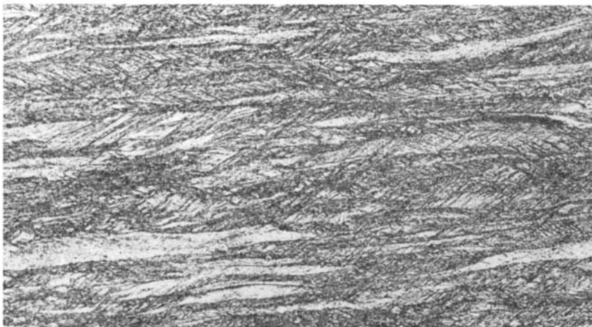
ELONGATED GRAINS appear in brass after it has been deformed by cold-rolling to a decrease in thickness of 75 percent. Distortion of the crystal lattice makes each grain stronger.
