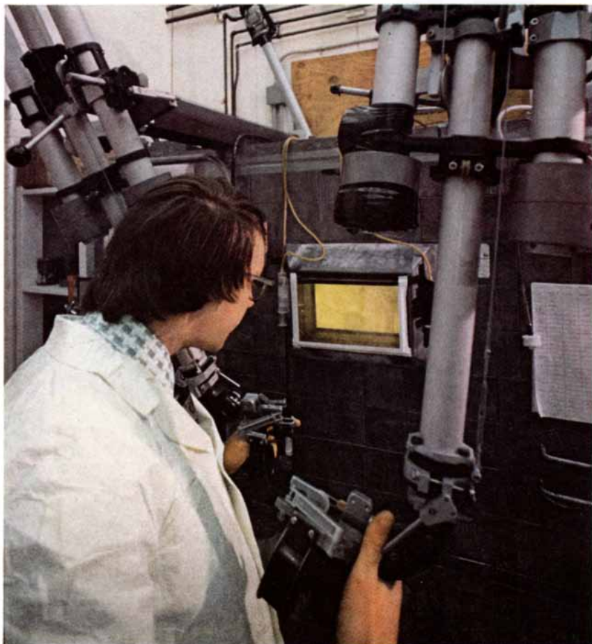
After high-energy deuteron bombardment, a radioactive magnesium target is handled inside a "hot" cell at NEN's North Billerica, Mass. facility.
