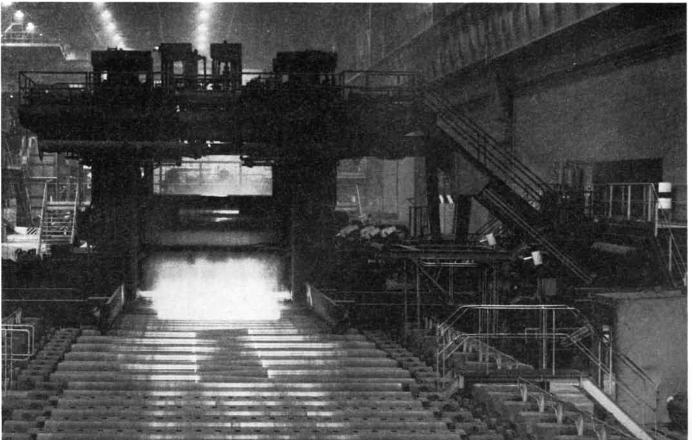
Steel Works of the United States Steel Corporation. This mill can roll plates of from 30 to 200 inches in width and from 3/16 inch to
