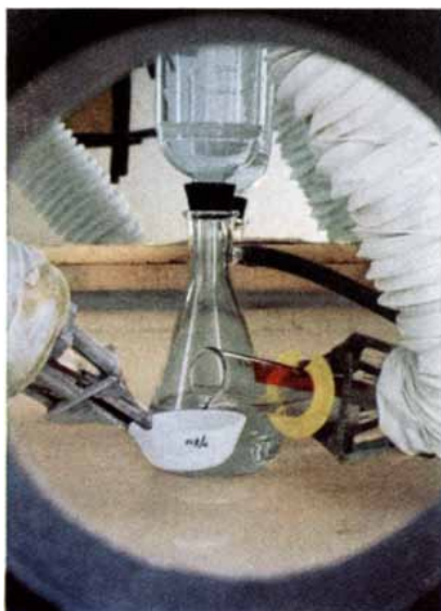
Inside a "hot" cell, ^{22}\text{Na} in solution is transferred to a teflon vessel before evaporation.
