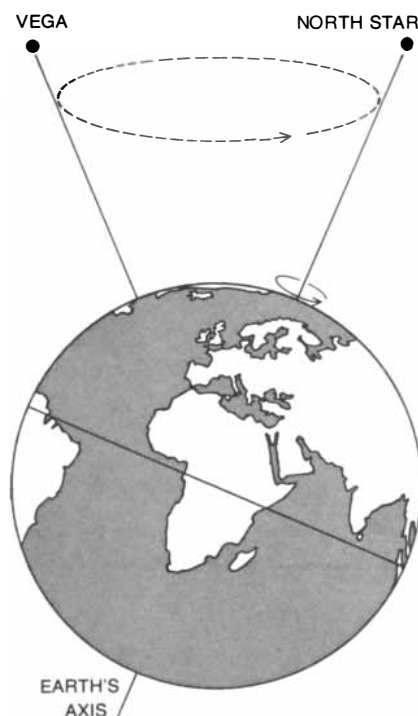
PRECESSION OF EARTH'S AXIS produces change in the apparent position of the stars. In 13,000 years, as the polar axis moves through half of its circle, the star Vega will become the new polestar and the present North Star will shift to 43 degrees north.
