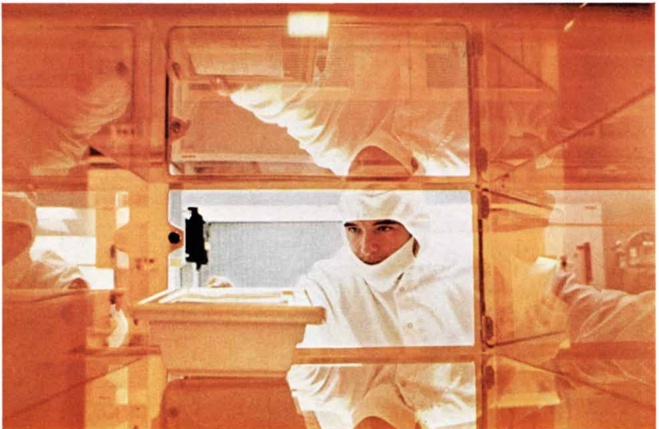
At the IBM Systems Product Division in East Fishkill, N.Y., a technician wearing a special sterile suit treats silicon wafers with a light-sensitive chemical used in the etching of circuits. The circuits were designed with ASTAP, a simulation tool.
