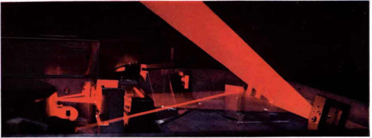
In the 3800 printer, the low-power laser beam shown here sweeps across a drum (not shown) coated with photoconductive material and exposes only the areas to be printed.
