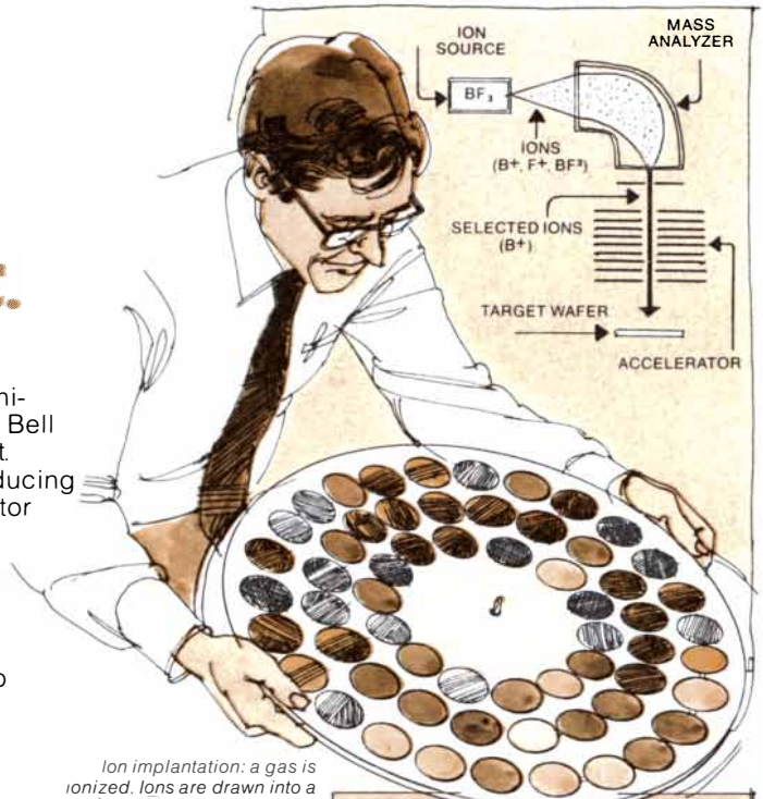
With the rotating mechanical scan method, a 3-inch silicon wafer can be implanted in a few seconds. Conventional x-y mechanical scans require about a minute.
