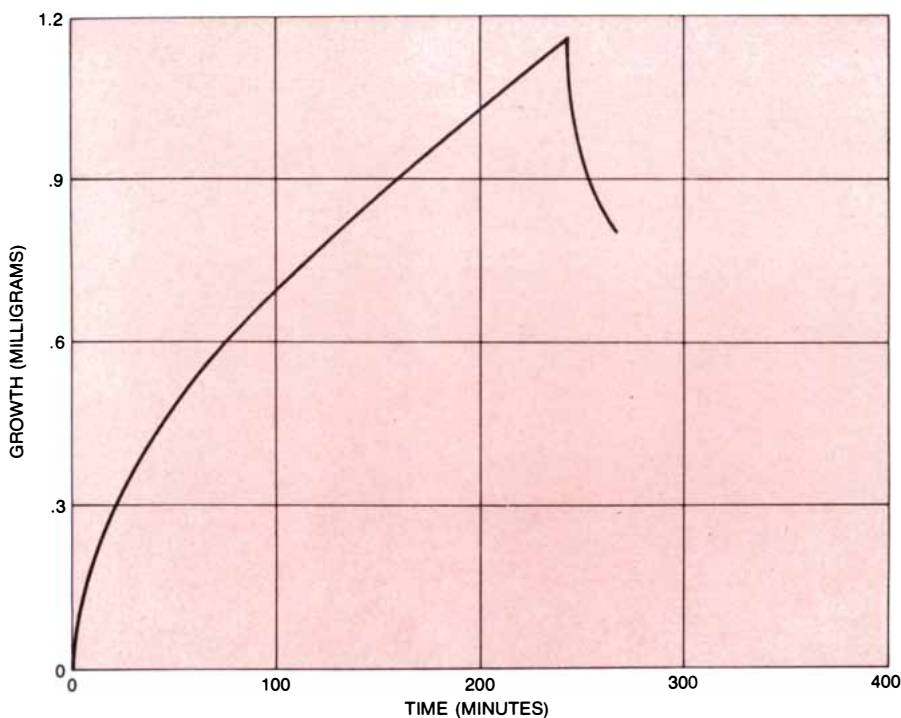
SINGLE BUILDUP CYCLE in the authors' apparatus is charted. The conditions in the apparatus were a temperature of 1,020 degrees C. and a methane pressure of .07 torr. During the four hours of the cycle the gain in weight of diamond was about 2.7 percent. The point at which the curve drops represents the time when air was admitted to the reactor for the purpose of removing graphite, which invariably accumulates during synthesis of diamond.
