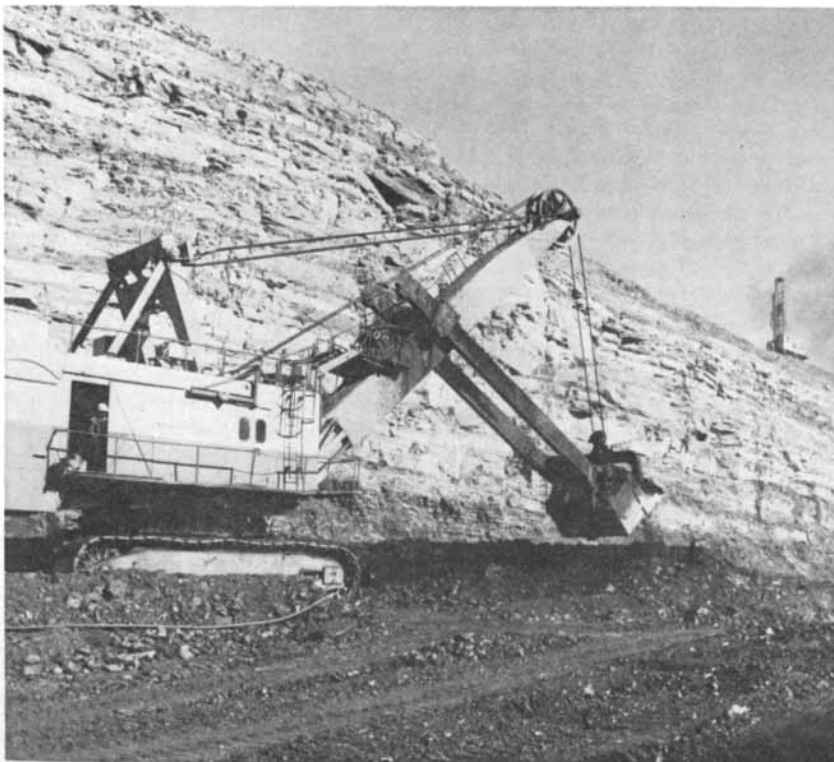
REMOVAL OF COAL proceeds at the Black Mesa Mine. At left a large power shovel digs coal from the seam and stands by to load it into a haulage truck. The rock wall with the drilling machine at its lip ( far right ) is the overburden that must be removed from coal.
