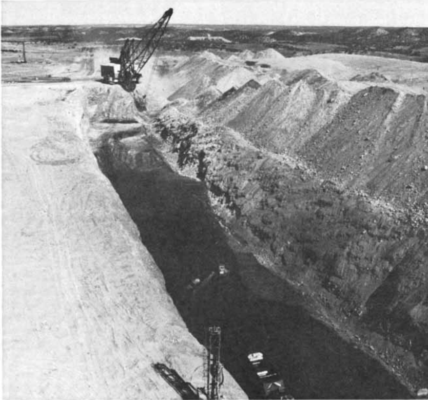
STRIP-MINING OPERATION is shown at the Peabody Coal Company's Black Mesa Mine in Arizona. At top a dragline removes overburden from the coal seam. The seam is visible in the trench below the dragline, as are two large trucks that haul the coal out of the trench. At bottom center is a drilling machine employed to prepare the overburden for blasting.
