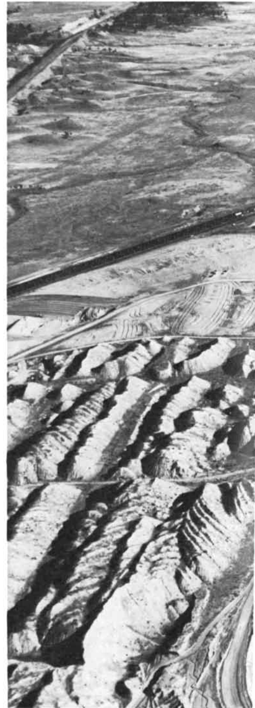
STRIP COAL MINE is operated by the Western Energy Co. at Colstrip in southeastern Montana. The prominent ribbed ridge at lower right is a spoil pile made up of ma-
