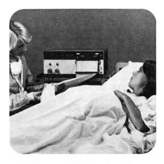
clearly identify the type of measurement method in use. An acceptance lamp lights with every valid heart rate measurement, and an INOP indicator immediately signals if there is any problem in the ECG electrode or transducer.
