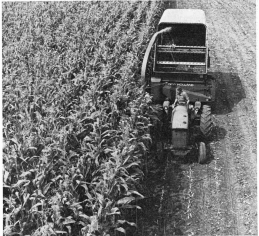
CORN IS HARVESTED for silage. Corn ( Zea mays ) is a member of the grass family and an annual plant. The harvesting machine being towed by the tractor cuts the corn near the base of the stalk and then chops the entire plant into the fine material that is being blown into the forage wagon. Corn serves both as a forage and as a major feed grain for livestock.
