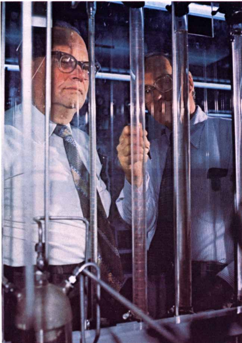
At Mobil's Paulsboro Research Laboratory, Dr. C. Dwight Prater (left) and Dr. Vern W. Weekman Jr., check the latest catalyst aging run as methanol is converted into gasoline.
