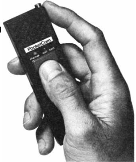
The PocketCom measures approximately 3/4" x 1 1/2" x 5 1/2" and easily fits into your shirt pocket. The unit can be used as a personal communications link for business or pleasure.
