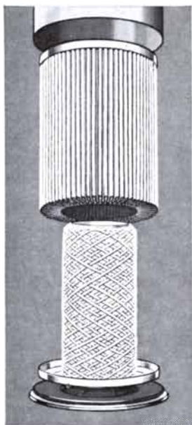
The outer filter: a 6 foot phenolic impregnated cellulose element. The inner filter: a fiber strand more than 60 feet long, wound on a steel core. Your oil goes through both approximately once every 30 seconds!
