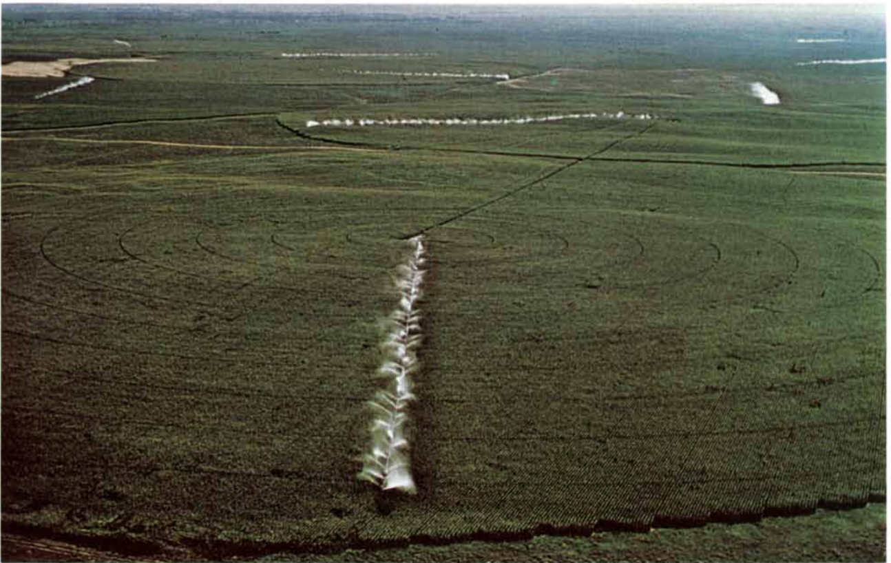
OBLIQUE AERIAL VIEW of a quarter-section circular cornfield in Nebraska shows how in the center-pivot irrigation scheme water is applied automatically by means of a series of sprinklers of the impact
