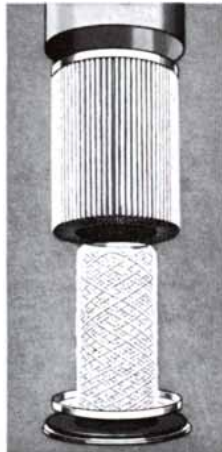
The outer filter: a 6 foot phenolic impregnated cellulose element. The inner filter: a fiber strand more than 60 feet long, wound on a steel core. Your oil goes through both approximately once every 30 seconds!
