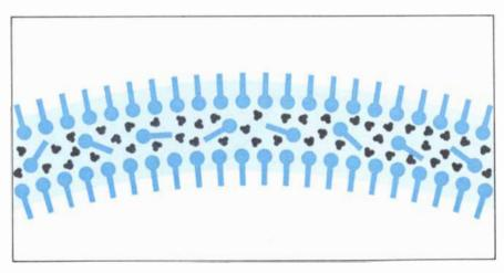
SECOND IMPORTANT EFFECT of soap on the formation of a liquid film is to limit the thinness of a film made from soapy solution to the length of two soap molecules stacked end to end.
