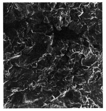
SPONGELIKE MICROSTRUCTURE of directly reduced iron appears in this micrograph of a pellet. Enlargement is 600 diameters.
