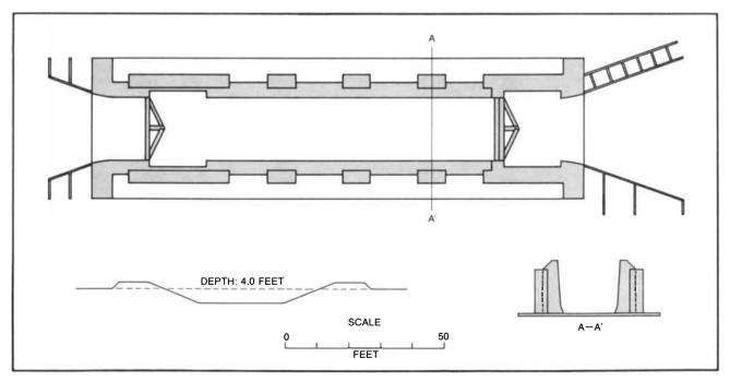
LOCK ON THE ERIE CANAL (top) and profile of the canal bed (bottom) are shown to the same scale in these simplified drawings based on contemporary plans. The V formed by the paired gates at each end of the lock points upstream; water pressure keeps the gates
