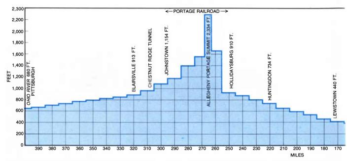
PENNSYLVANIA CANAL PROFILE shows a 2,334-foot lift from sea level at Philadelphia to the summit of the inclined-rail system con-
