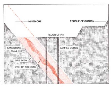
ORE BODY AT OKLO, shown in a schematic profile of the mine, lies above a sandstone wall with an average slope of about 45 degrees. The reactor zones are within the rich vein of ore, which is roughly a meter thick. The zones generally have a lenticular cross section. The extent of the ore body and the location of the reactor zones were revealed by removing core samples.
