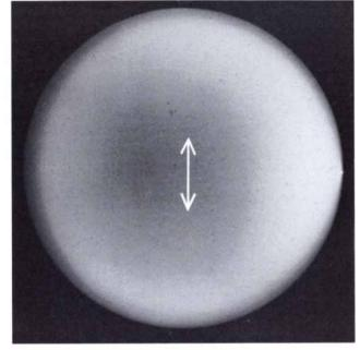
the polarizing filter is parallel to the solar meridian. When the axis is perpendicular (right), however, variation in intensity disappears.
