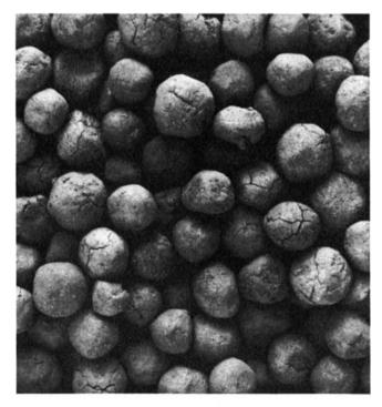
IRON PELLETS manufactured by the Midrex direct-reduction process at Sidbec plant are from two to three centimeters in diameter.
