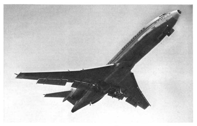
A Boeing 727 shortly after takeoff, with its triple-slotted trailing-edge flaps extended, from Handling the Big Jets
