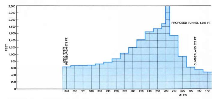
CHESAPEAKE AND OHIO PROFILE, as proposed, shows a lift from water level at Washington to 1,898 feet, where a four-mile tun-
