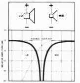
Diagram A. When drivers are placed in-phase, a problem of audible "suck out" is created.
