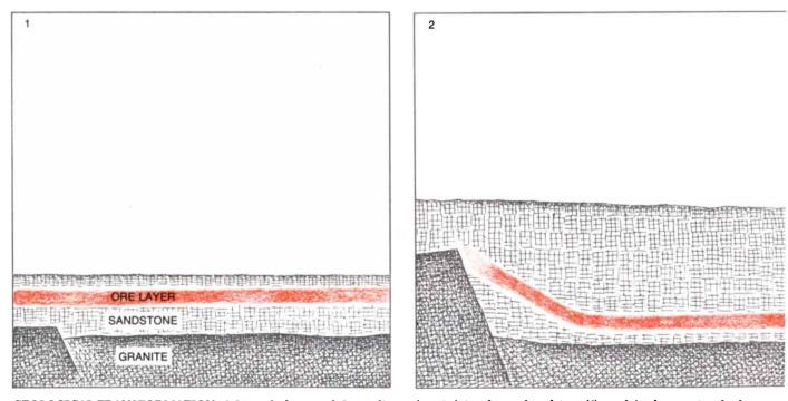
GEOLOGICAL TRANSFORMATION of the ore body created the conditions necessary for the operation of the natural reactor and preserved the evidence of the reaction for almost half the life of the planet. After the ore had been deposited in the river delta it was compacted along with other sed-
