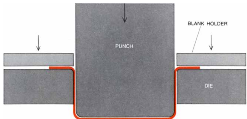
DRAWING , one of the two major modes of forming metal by stamping, is illustrated by the deep drawing of a cylindrical cup. The circular blank is drawn into the cup-shaped die by the flat-headed punch. The wall of the cup supports the major part of the load and tends to undergo thinning. Best material for drawing is therefore a material that is resistant to thinning.
