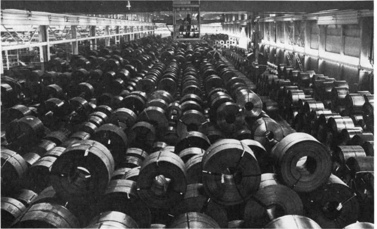
COILS OF SHEET METAL that will be formed into parts for automobiles are stored at a plant of the General Motors Corporation. The metal is low-carbon steel. Coils are transported to an adja-
