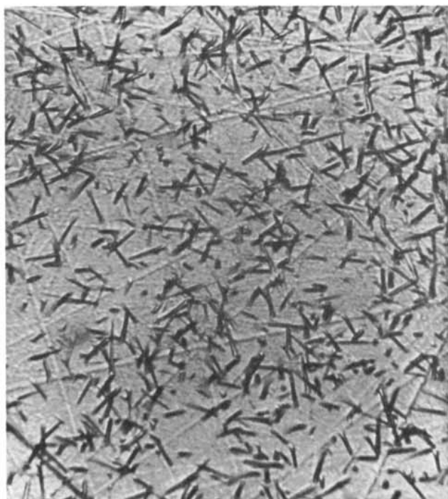
ANNEALING BY HEAT causes fission tracks to disappear as the disruption of the crystal lattice mends. An etched section of an apatite
