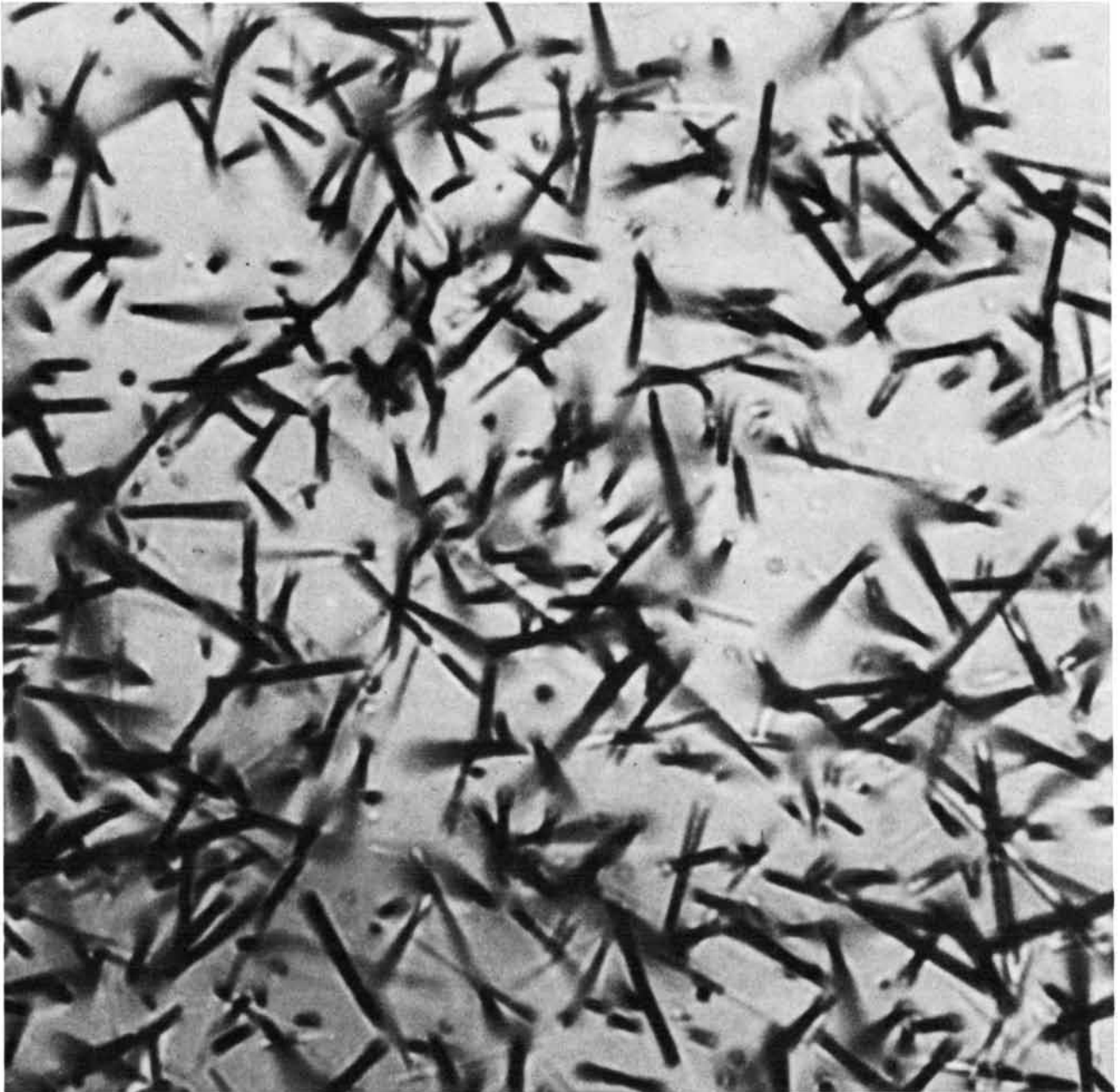
FISSION TRACKS in a crystal of zircon appear in this light micrograph. The magnification is 3,100 diameters. Visibility of the tracks has been enhanced by an etching process that increases the diameter
