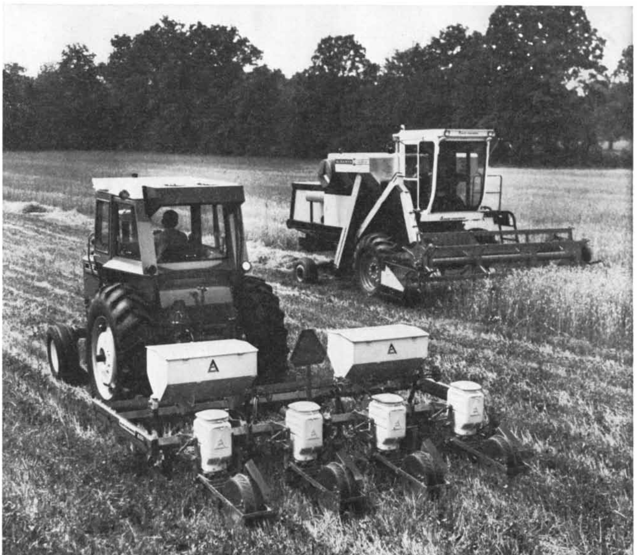
MULTIPLE CROPPING is made possible on a farm in Ohio by planting without tillage. The machine at the right is harvesting a crop of wheat as the machine at the left plants soybean seed in the wheat stubble. The two larger white containers on the planting machine
