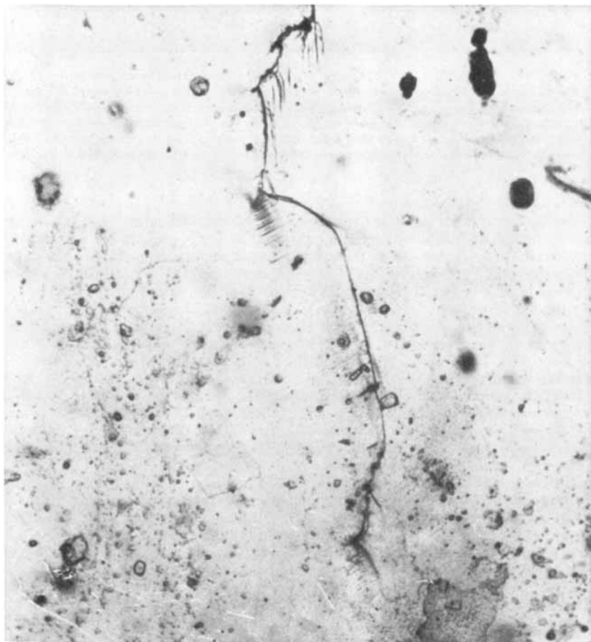
FATIGUE CRACK IN ALUMINUM looks like this in an optical microscope. Although optical and other standard imaging techniques are usually effective in revealing cracks and other surface flaws, they give no information about how recent they are or how they are progressing.
