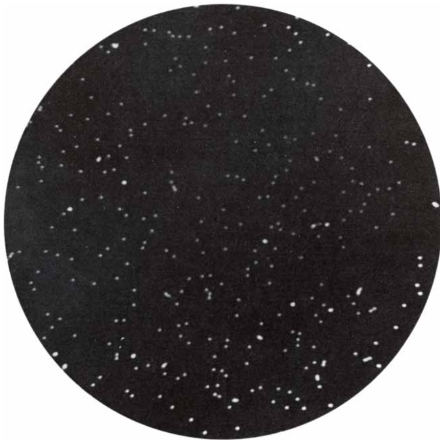
SPECIAL STIMULUS employed by the authors in their laboratory to study the perception of motion under controlled conditions consists of a moving pattern of small, bright dots electronically generated on the screen of a cathode-ray tube with a computer. To an observer the stimulus looks like an infinitely large sheet of random dots moving behind a stationary aperture.
