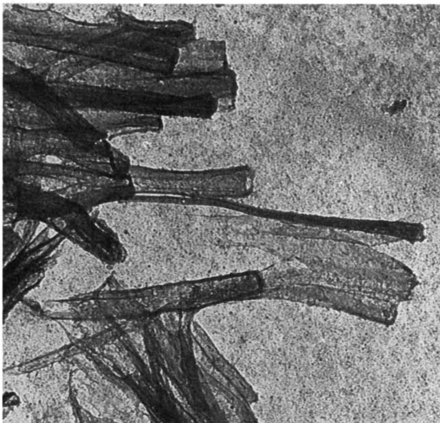
HYDRATED PORTLAND CEMENT is seen in microstructure in the transmission electron microscope. The top micrograph shows a wet sample of cement after some two days of hydration; one can see a well-developed fibrillar growth of silicate gel around the cement grains. The enlargement is 20,000 diameters. The bottom micrograph (enlarged 70,000 diameters) shows a dried sample of hydrated cement that clearly exhibits the tubular nature of the fibers.
