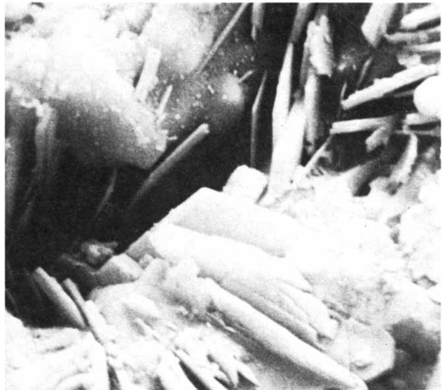
HIGH-ALUMINA CEMENT , which was designed to resist attack by sulfates and which hardens faster than portland cement, is portrayed at the same magnification as the micrograph at the top of the page. The reaction products are crystalline aluminates with an interlocking platelike and needlelike form. The chemical instability of these reaction products is the cause of a problem with high-alumina cement, namely the unpredictability of its long-term strength.
