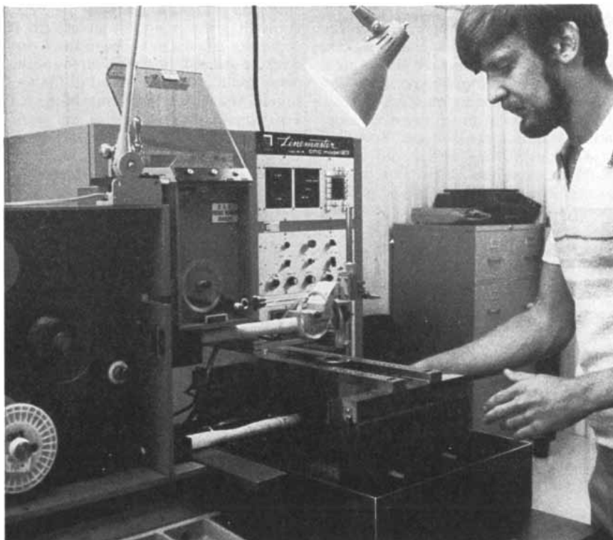
NUMERICALLY CONTROLLED MACHINE TOOL ( foreground ) is computer-programmable. In the background is the keyboard and memory component; programs for various tasks are entered and called up as needed. Seen at work at the Wilsey Tool Company, Inc., of Quakertown, Pa., the tool does electric-discharge machining; a moving wire is the electrode. It is made by Andrew Engineering of Hopkins, Minn. Its cutting face appears in the photograph below.
