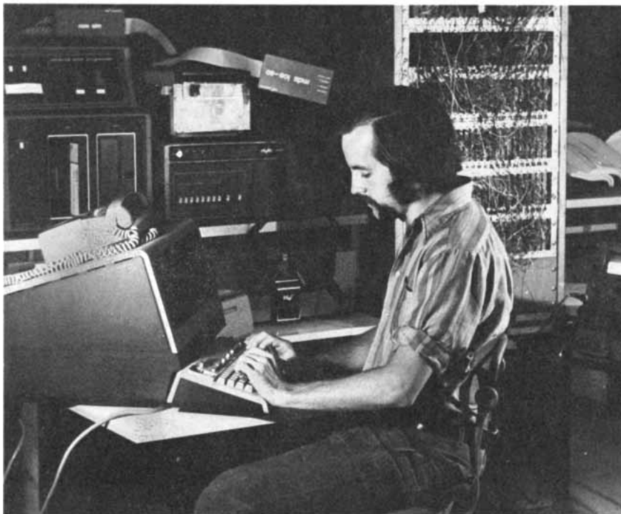
MICROPROCESSOR SYSTEM DEVELOPMENT is studied in the author's laboratory at M.I.T. The development engineer is working at a terminal tied into a full development system of the kind described in the illustration on the next two pages. The microcomputer itself, an Intellec MDS-80, is in the cabinet at the rear immediately to the left of the engineer's head. Directly under the microcomputer is a paper-tape reader. To the left of the microcomputer is a dual floppy disk, and above it is a PROM programmer. The software facilities available to the engineer can be extended beyond full development system to include complete software capabilities of a minicomputer in "Triad" system depicted in upper illustration on page 156.
