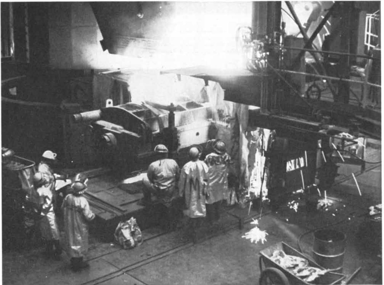
CONTINUOUS CASTING OF STEEL SLABS calls for a complex automatic routine of water-cooling. This machine is the constant-radius continuous-strand caster at the Burns Harbor, Ind., complex of the Bethlehem Steel Corporation; the slab is more than six feet
