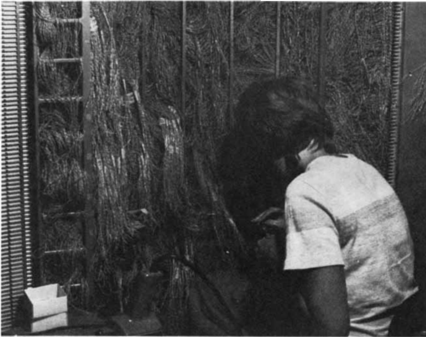
THICK MAT OF WIRES covers the back panel of a large general-purpose computer, in this case the Cray Research, Inc., CRAY-1. Moving data over the wires takes time and costs money, and the thickness of the mat makes repairs difficult. Arranging elements of a computer so that wires are all parallel would greatly reduce the complexity and thickness of the mat.
