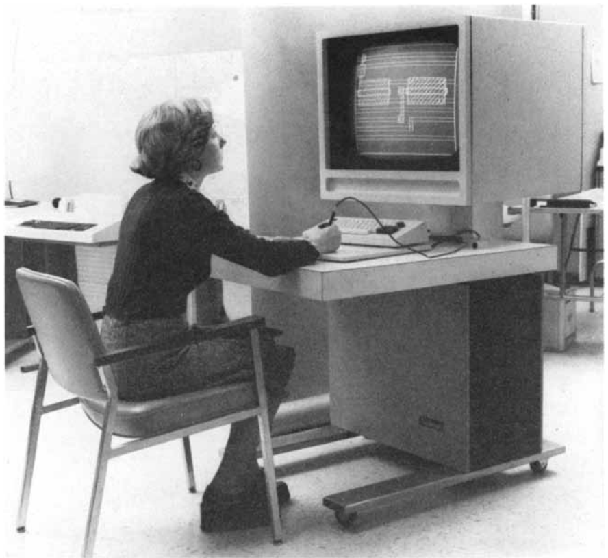
MICROCIRCUIT IS LAID OUT with the aid of a computer. The portion of the large-scale integrated circuit being laid out in this demonstration is studied by the circuit designer on the screen of a cathode-ray tube. By typing in commands or redrawing with a "light pen," circuit elements can be added, subtracted or moved. The terminal seen here is made by Applicon Inc.
