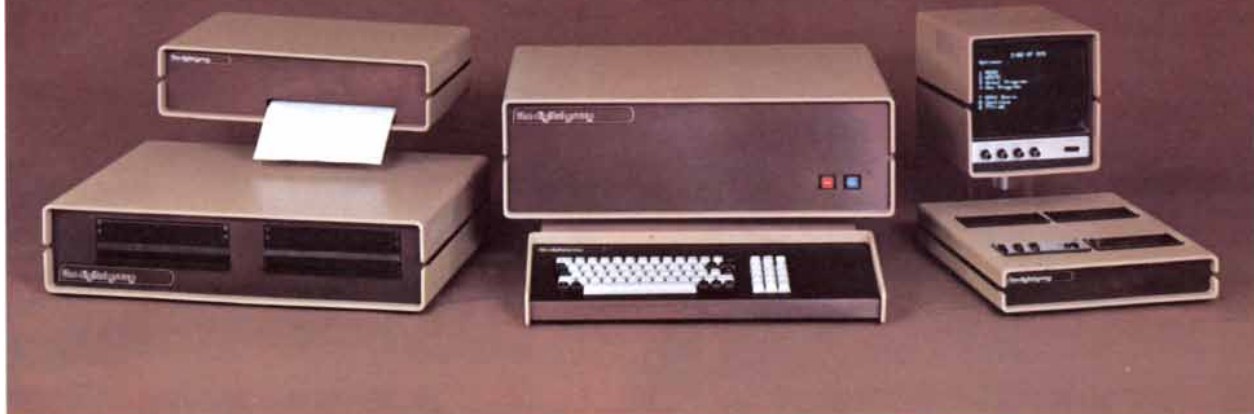
Clockwise from top left: Impact Printer, CPU, 9" Video Monitor, Cassette Storage System with Four Drives, Keyboard, Dual Floppy.
