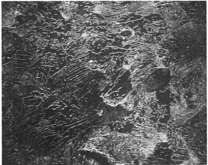
PEARLITE , a characteristic microstructure of carbon steels, has a layered pattern at high magnifications. This scanning electron micrograph enlarges the sample 1,250 diameters. It shows a gold-covered replica of the corroded surface of a steeled-iron blade found at a site in Israel: Tel Fara South. Although the iron is oxidized a relic pearlite microstructure is preserved. The blade was made available for study by the Institute of Archaeology of the University of London.
