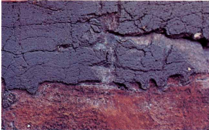
MANGANESE AND IRON minerals were brought up from the West Indian Ocean in 1976 by the research vessel Vema , operated by the Lamont-Doherty Geological Observatory. In this sectioned and polished specimen the gray metal is manganese oxide and the reddish metal is iron hydroxide. The deposit was found 4,000 meters below sea level in a fracture zone near the axis of the Mid-Indian Ridge, a spreading center. It is a hydrothermal deposit: its metals were leached from the crustal basalt by circulating seawater and brought up through the sea floor at a hot spring. When such a hot solution enters the cold oxygenated water of the sea floor, metals such as iron and manganese tend to be oxidized and deposited. Iron and manganese separate because iron is less soluble than manganese in seawater and so may be deposited first.
