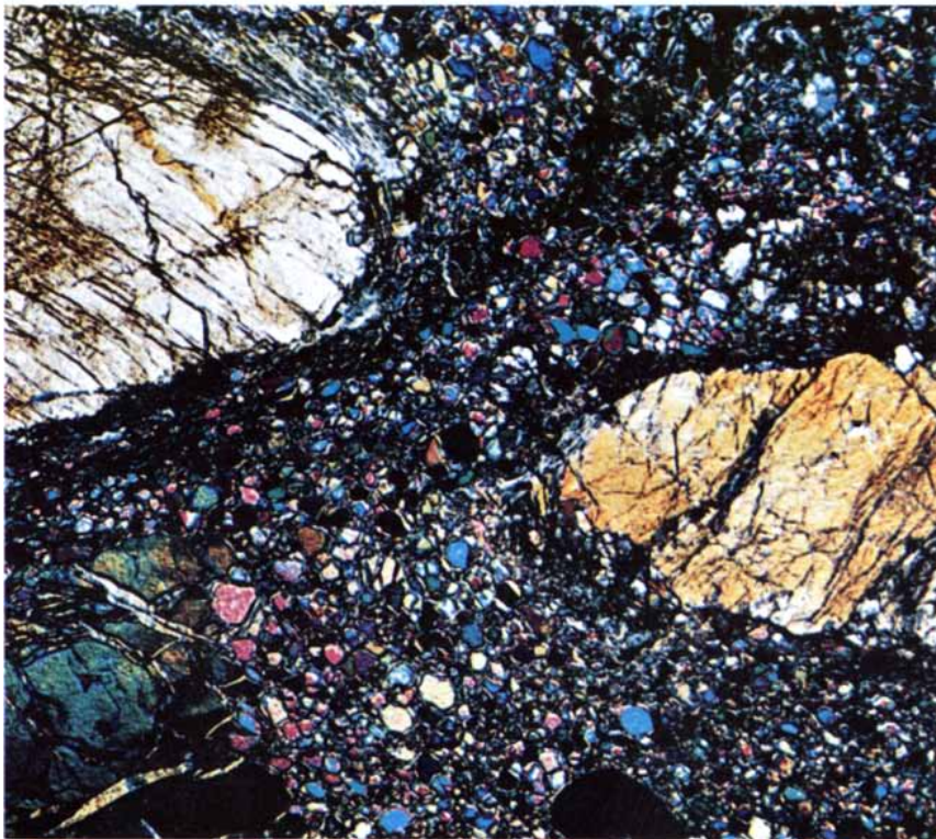
SHEARED NODULE is seen in a photomicrograph made between crossed polarizing filters in order to enhance contrast between crystals. The large crystals are orthopyroxene. They are set in a matrix of olivine that has been reduced to a finely milled powder by extreme deformation. The specimen is from the Bultfontein pipe at Kimberley. It is magnified some 20 times.
