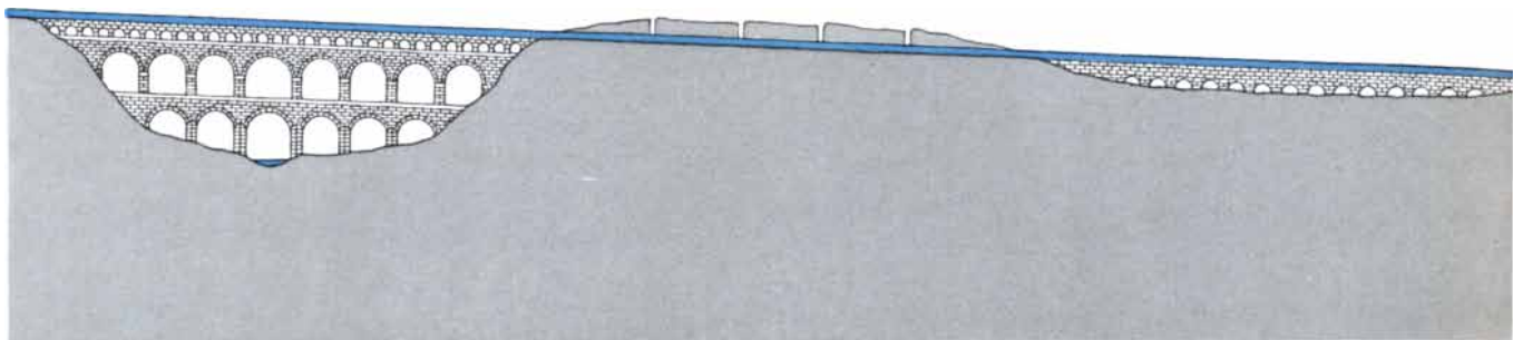
CONTINUATION OF AQUEDUCT shows the water being carried first across a fairly deep valley (up to 150 feet) by a three-tier bridge. (The Pont du Gard, a three-tier bridge, survives in France.) There-
