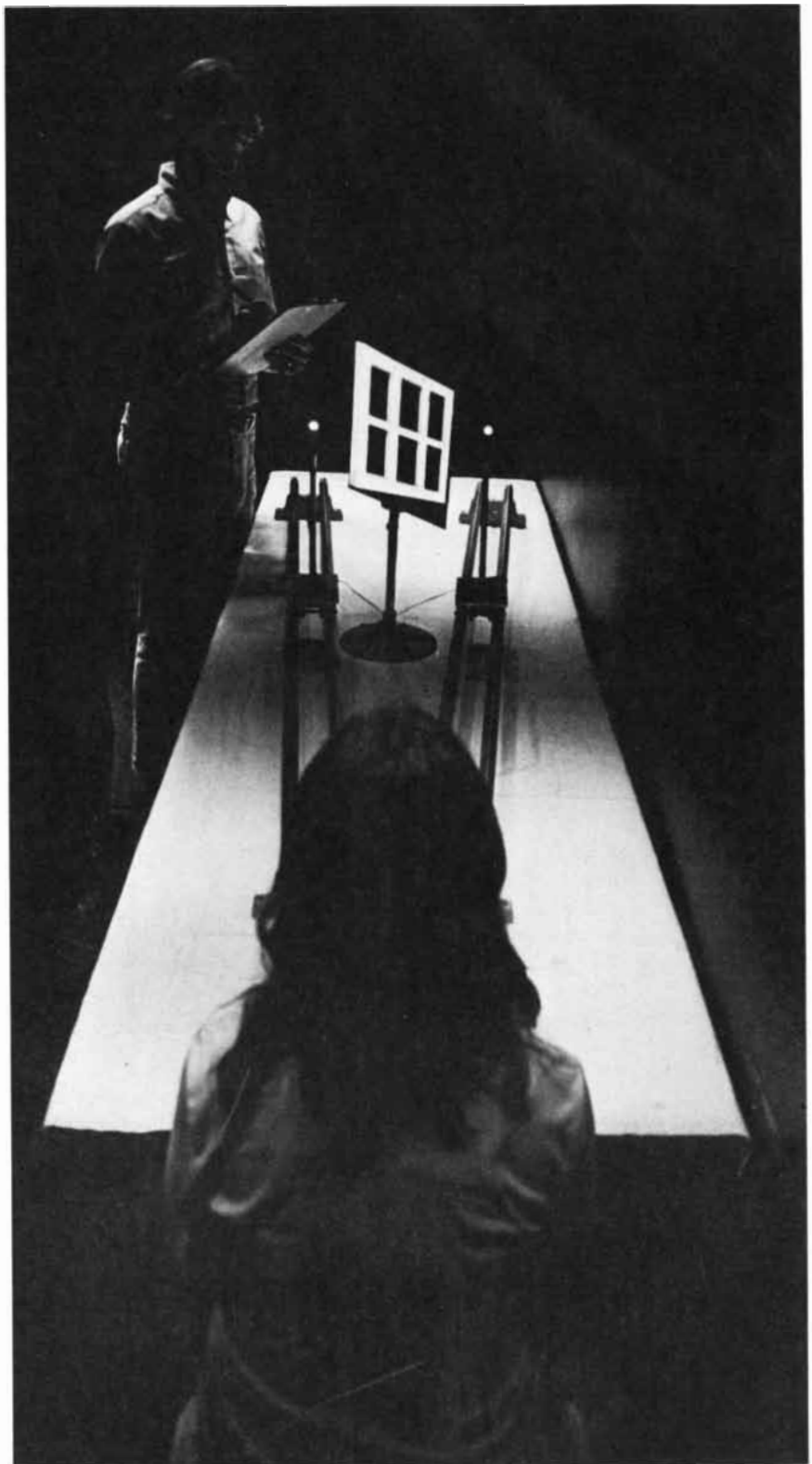
SPATIAL ADJACENCY EFFECTS are demonstrated when a trapezoidal window, made by masking and shading portions of an electroluminescent panel, and two luminous disks are viewed binocularly in an otherwise dark visual field. One end of the window (here the right end) is closer than the other, but perceptually it is farther away. The perceptual error is transmitted to the disks. They are physically equidistant from the observer, but perceptually the right disk is beyond the left one. If the disks are moved along the tracks together, they appear to move at different speeds while they are in the vicinity of the window. The influence of the window on their perceived position (and motion) diminishes as they move away from it. (The window's downward slant here results from the angle at which the photograph was made.) Application of the adjacency principle to these phenomena is illustrated in diagram on page 136.
