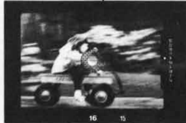
The electronic viewfinder: light emitting diodes tell you what the camera is doing automatically to give you correct exposure.
