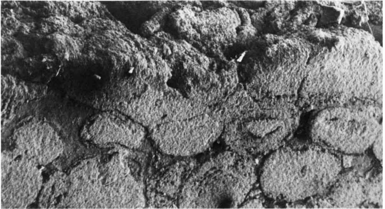
WEATHERED PORTLAND LIMESTONE from St. Paul's Cathedral in London is shown in a scanning electron micrograph at an enlargement of 120 diameters. In the upper part of the micrograph one sees an area near the surface of the stone; the lower part is the interi-
