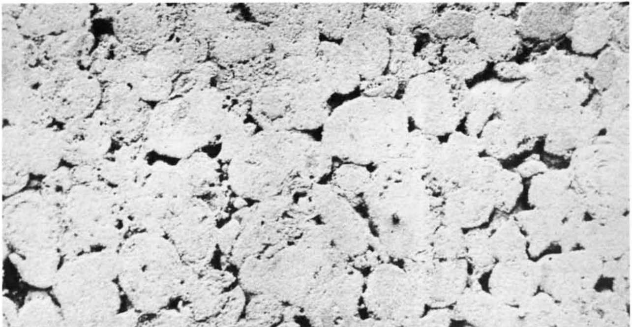
DEEPER SECTION of the limestone from St. Paul's Cathedral is enlarged 40 diameters in this scanning electron micrograph. The open
