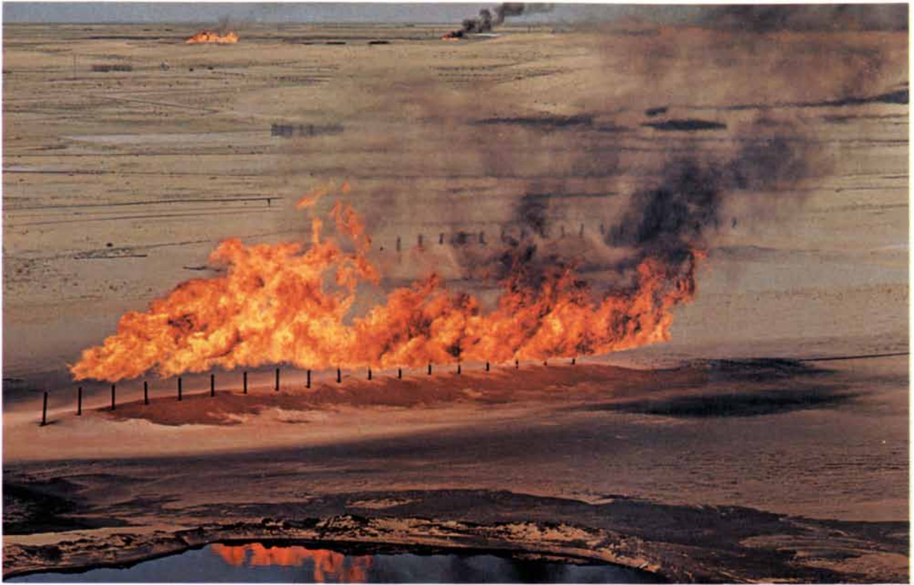
GAS FLARES ARE SPREAD over a large area in remote regions in order to ensure complete combustion. This photograph, made from the vantage point of a nearby drilling rig, shows such a flame at an oil
