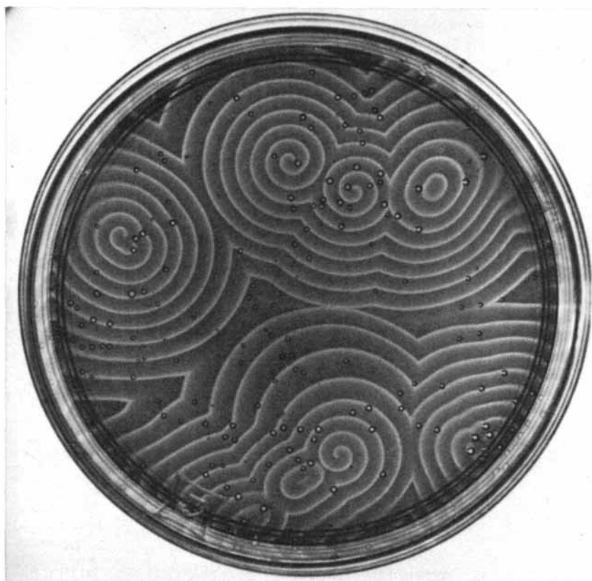
Spiral-wave patterns in an unstirred Winfree mixture
