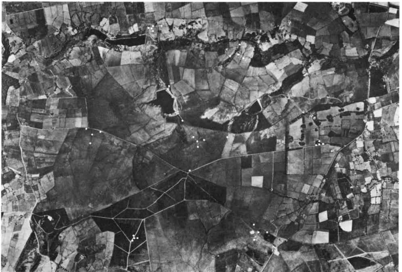
AIR SHOWERS ARE DETECTED by a giant array of detectors mapped by the dots on this aerial photograph of Haverah Park outside Leeds in England. The diameter of the roughly hexagonal area covered by the detectors is about four kilometers. Each detector is
