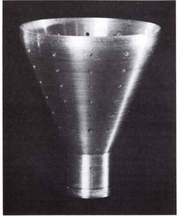
fits snugly into cone at the right when they are fastened with a screw through their apexes. Two small holes in the outer wall communicate with one larger hole in the inner wall through the grooves in the surface of smaller cone. Model is seven centimeters high and five wide.
