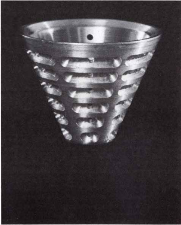
MODEL OF AN ARCHAEOCYATHID was made out of aluminum by William L. Balsam and the author at Duke University to enable them to test whether the animal was the right shape to take advantage of induced flow. In the assembled model the cone at the left
