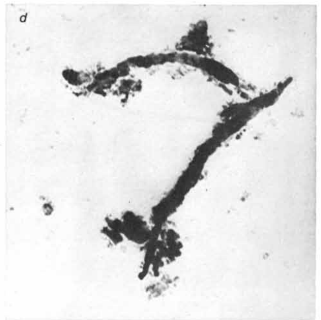
(b) or abraded (c) have the same characteristics but are smaller and more irregular. The particles removed when copper is polished (d) are even smaller, but they are undoubtedly ribbons and seem to have the periodic structure typical of a machining chip. Evidently grinding, abrasion and polishing are all similar abrasive-machining processes. Enlargements are respectively 90, 520, 472 and 70,800 diameters.
