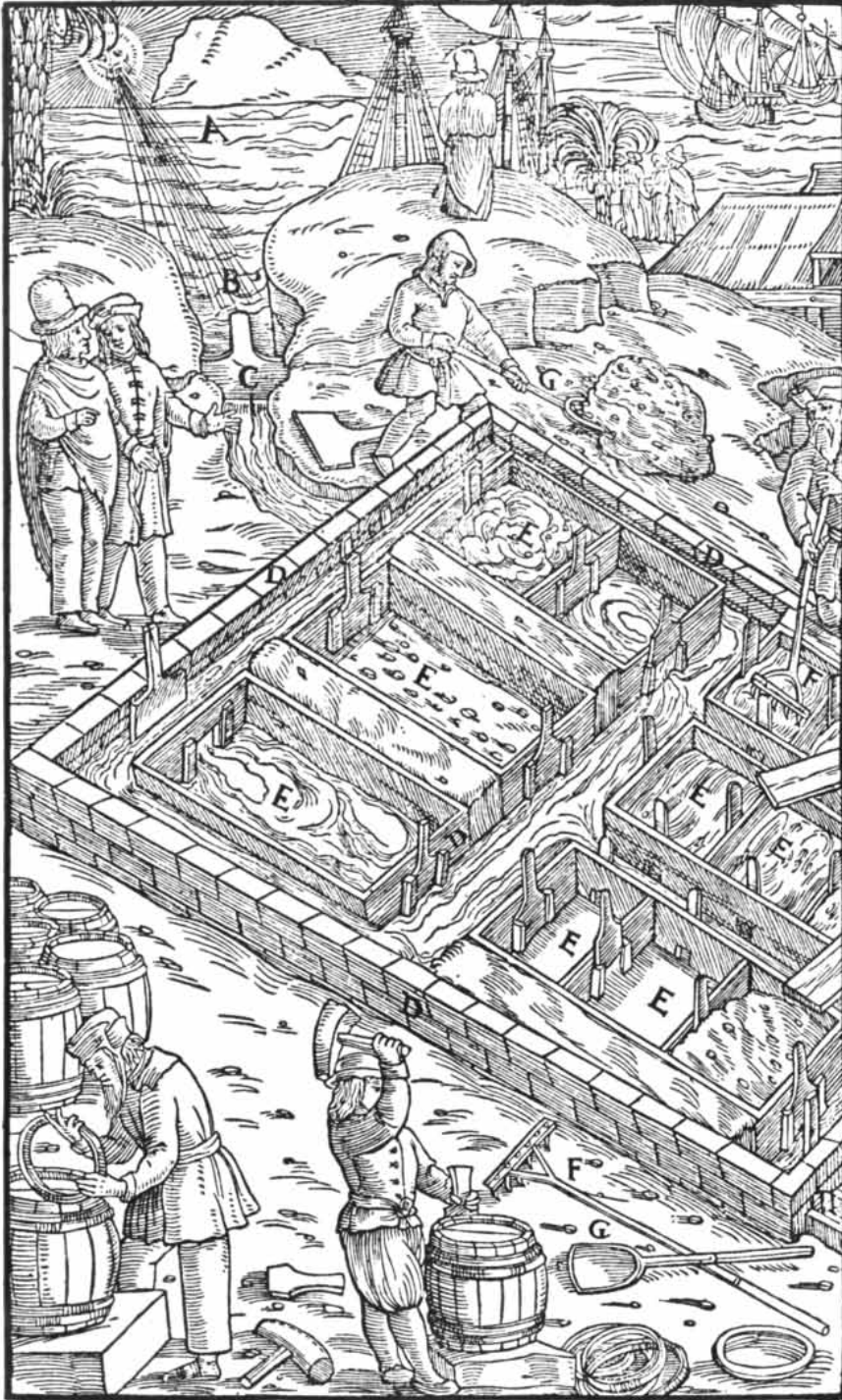
SALT IS MADE FROM SEAWATER in this woodcut from Georgius Agricola's De re metallica of 1543. A is the sea, B a pool, C a gate, D trenches, E salt basins, F a rake and G shovels.
