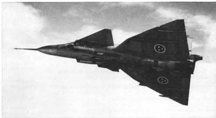
MODERN AIRCRAFT with an elevator in front is the Swedish Viggen, a short-takeoff-and-landing aircraft with a speed above Mach 2. Such a configuration is known today as a canard.
