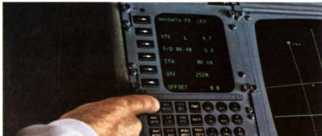
Flight management control panel.
