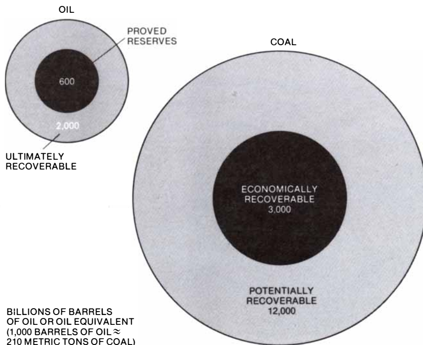
COMPARISON OF OIL AND COAL RESERVES shows that the world supply of potentially recoverable coal is equivalent to some 12,000 billion barrels of oil, or six times the estimated reserves of ultimately recoverable oil. The amount of coal that is economically recoverable with today's technology and prices is considerably smaller, equivalent to about 3,000 billion barrels of oil. Even this figure, however, is perhaps five times the proved reserves of oil.
