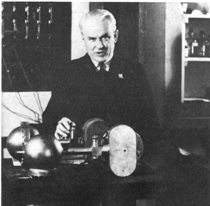
RECORDING ELECTROSCOPE displayed by Millikan in 1935 was a late model of the kind of equipment with which he had for years been studying ionization caused by cosmic rays.
