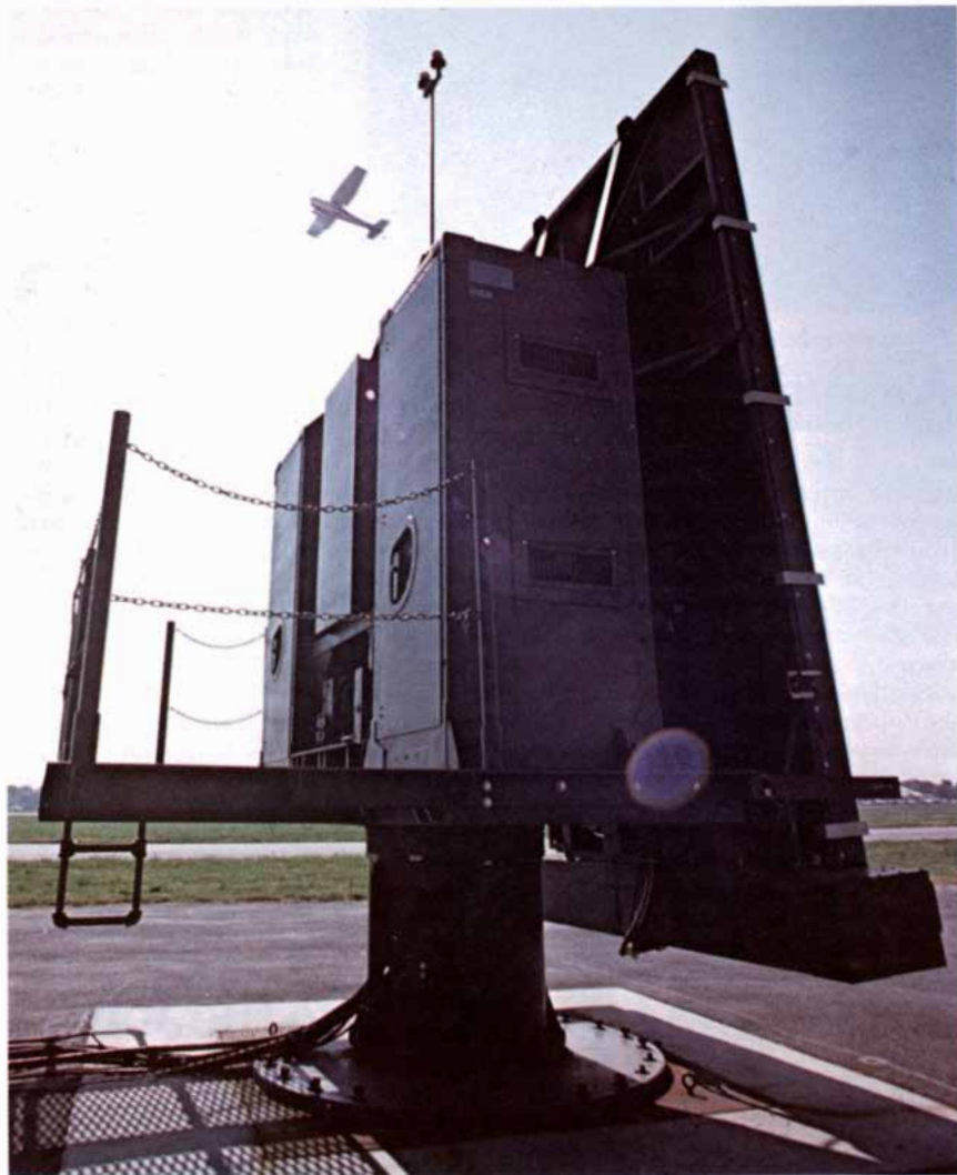
Prototype model of ITT Gilfillan PAR-80 phased array radar, which guides an aircraft through 20 miles of approach to a precise touchdown. Computer simulation played a major role in its design.
