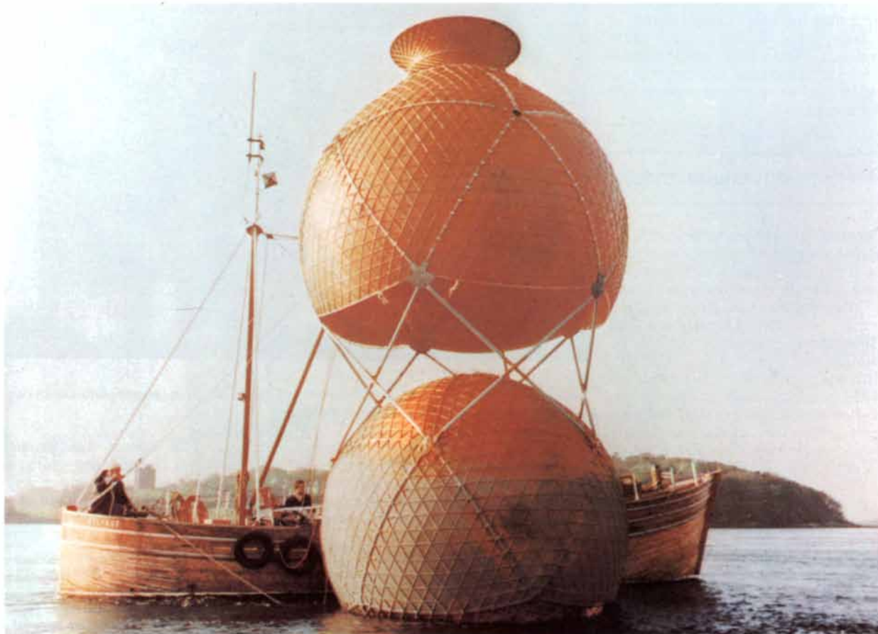
Wave-energy research by Queen's University, Belfast: when part-submerged, this one-tenth-scale hydropneumatic buoy harnesses wave motion to generate electricity through the piston action of water in the upper chamber.
