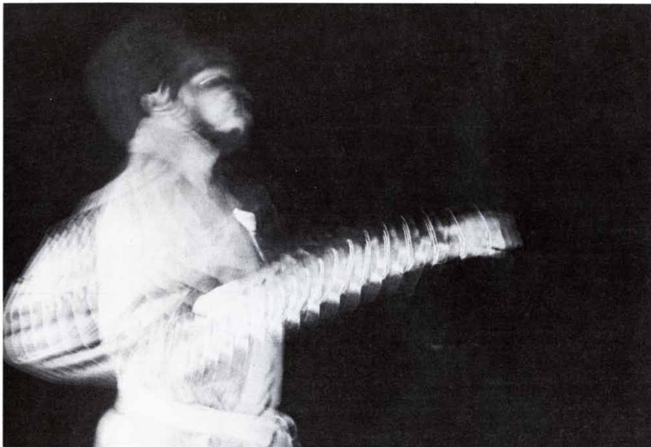
STROBOSCOPIC PHOTOGRAPH of a forward karate punch, in which the karate expert was illuminated by 120 flashes per second, indicates that the fist reaches maximum speed shortly before the arm
