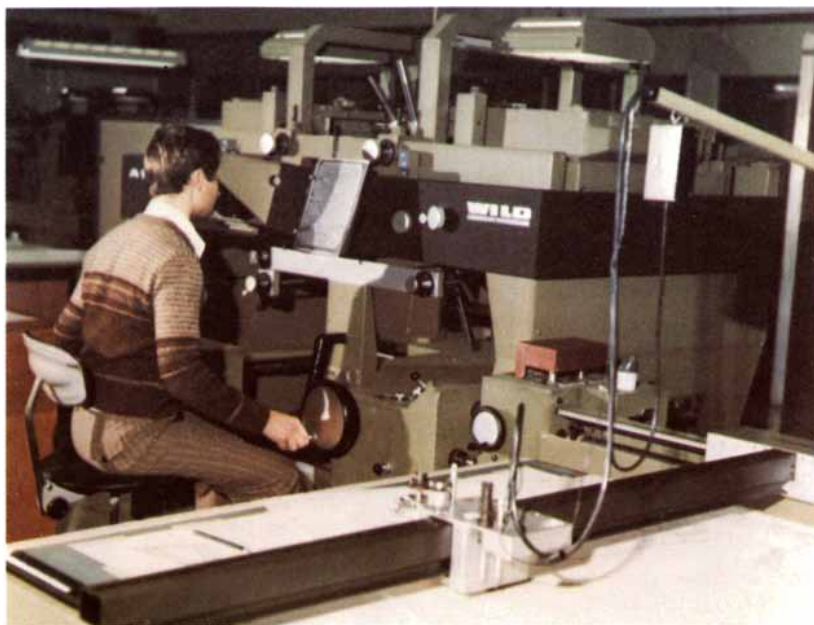
Photogrammetry at BKS Surveys, Coleraine: using stereo plotters, aerial photographs are translated into detailed maps of the areas surveyed.
