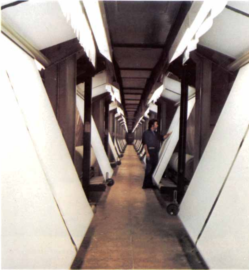
Woven cloth is inspected in the lower level of the weaving unit of Courtaulds' integrated textile plant at Campsie; the cloth is fed down from weaving machines on the floor above.
