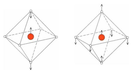
VIBRATIONS OF SULFUR HEXAFLUORIDE can be excited by infrared radiation. The molecule consists of a sulfur atom (*color*) surrounded by six fluorine atoms (*open circles*), which form the corners of an octahedron. For clarity sulfur-fluorine bonds are omitted. In one fundamental vibrational mode (*left*) the sulfur atom moves toward and away from two fluorine atoms that are 180 degrees apart. In a second mode (*right*) the sulfur atoms move in the opposite direction.
