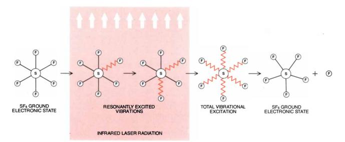
DISSOCIATION OF SULFUR HEXAFLUORIDE, shown schematically, is induced by the sequential absorption of 35 infrared photons from a carbon dioxide laser. The energy carried by the photons is transferred to the sulfur-fluorine bonds (*color*) of the molecule,
