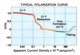
Our researchers have, in fact, determined all 10 steps that take place as  $Cr^{+6}$  reduces to bright Cr, pinpointed the step at which catalysis begins, and identified the active catalyst. (It's not the sulfate ion, as commonly held, but the bisulfate ion.)
