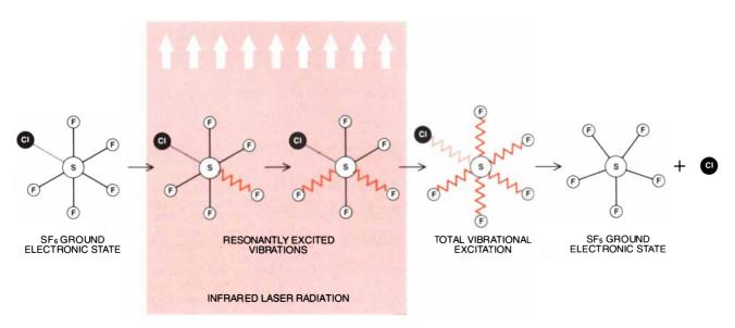
SUBSTITUTION OF CHLORINE ATOM for one of the fluorine atoms in sulfur hexafluoride yields  $SF_5Cl$ , a compound that can be used to clarify the mechanism involved in the laser dissociation of the molecule. If the laser is tuned to excite sulfur-fluorine bonds specifically, one would expect one of those bonds to break. Instead the
