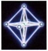
• Starting with  $Cr^{+3}$  fails because it immediately forms a stable complex with water molecules (see drawing) from which Cr cannot be deposited.
