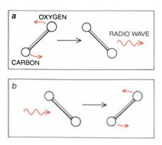
RADIO WAVE IS EMITTED by a molecule of carbon monoxide at a wavelength of 2.6 millimeters when the molecule stops rotating at the lowest speed allowed by quantum mechanics (a). The molecule can absorb radiation at the same wavelength by starting to rotate again at the identical minimum speed (b).
