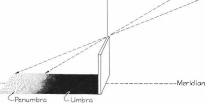
Gnomon method for determining the orientation of the sun's rays
