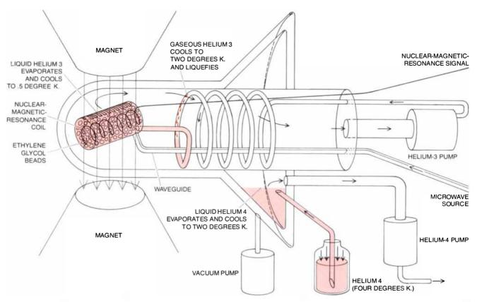
TARGET OF POLARIZED PROTONS is cooled to a temperature of .5 degree Kelvin, placed in a magnetic field of 25,000 gauss and exposed to microwave radiation that has a frequency of 70 gigahertz. The refrigeration is supplied by two isotopes of helium. The common isotope helium 4 cools the entire apparatus to two degrees K., and further cooling of the target itself is provided by the light isotope helium 3. Both cooling systems employ vacuum pumps to reduce the
