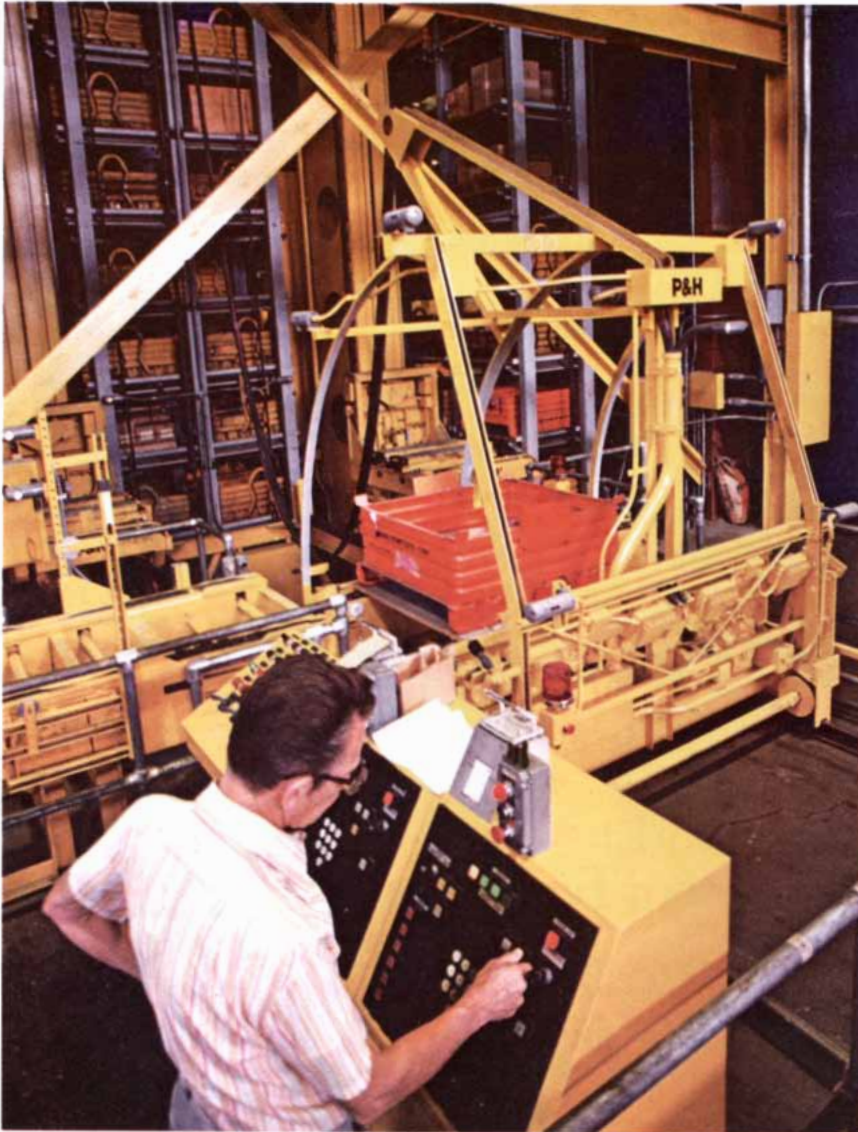
This automatic stacker crane travels to the selected bin and retrieves the required items. Computer simulation enables Harnischfeger to design efficient industrial material handling systems.
