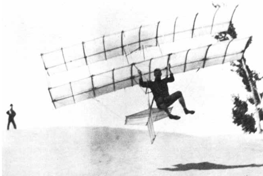
BIPLANE GLIDER was designed in 1896 by Octave Chanute, a civil engineer who was the most serious student of aeronautics in the U.S. before the Wrights began their work. They carried on a long correspondence with him, and he was on hand for many of their early flights. The pilot for this flight in 1897 in Indiana was A. M. Herring, one of Chanute's associates.
