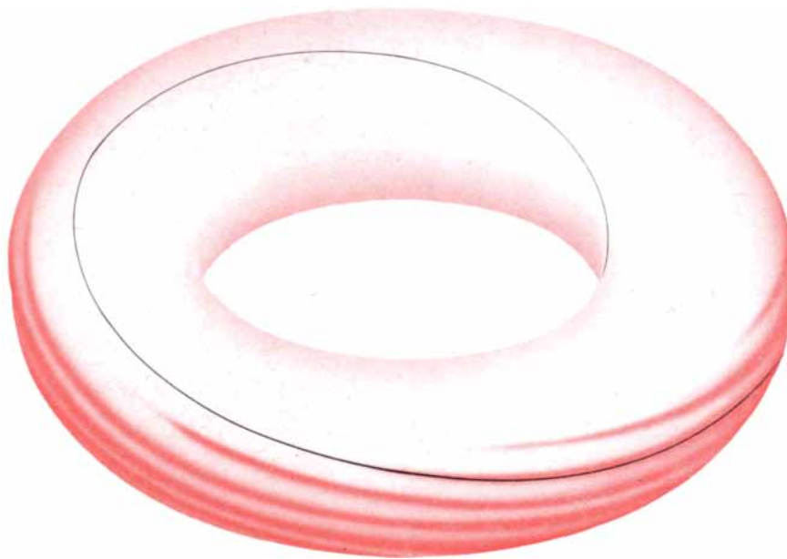
NEXT GENERATION OF PROBLEMS in tokamak research is expected to include a new class of macroscopic instabilities called ballooning interchange modes, one of which is illustrated here. In experiments with a high ratio of kinetic plasma pressure to magnetic-field pressure the plasma may have a tendency to squeeze out between the field lines of the magnetic bottle while deforming them slightly. The result in this case would be a ripple effect around the outside surface of the plasma torus, aligned approximately with the pitch of magnetic-field lines.
