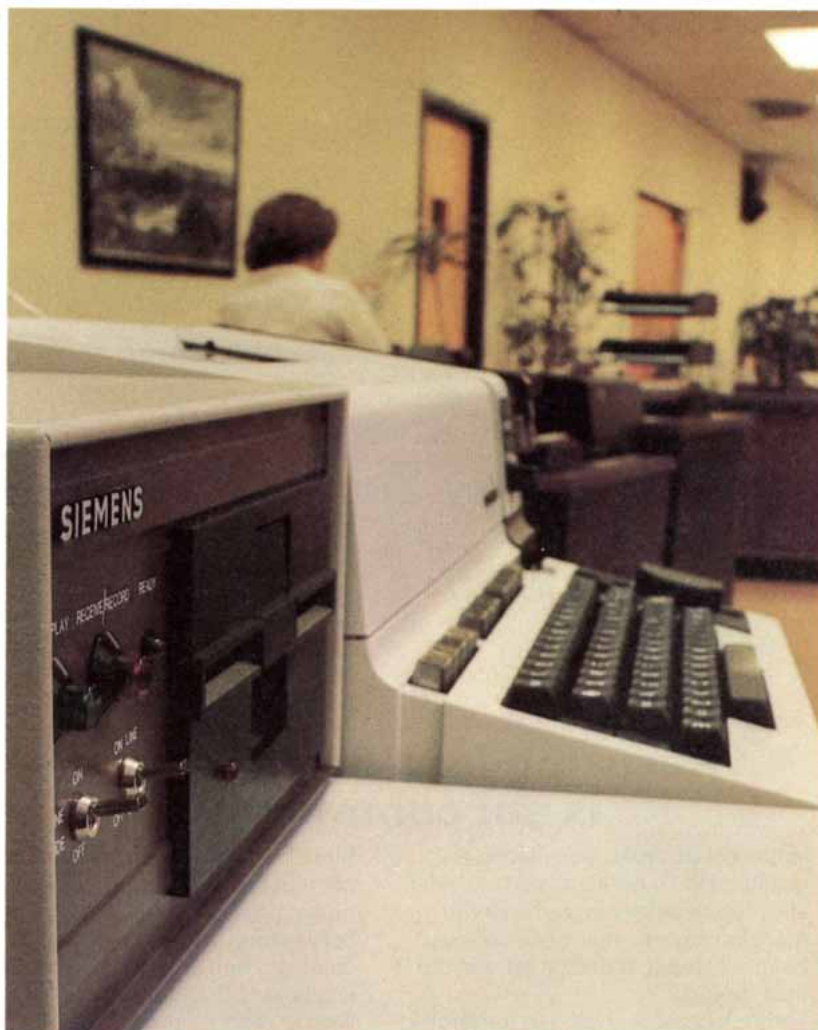
Siemens all-electronic teleprinter with mini-disk storage and editing unit.
