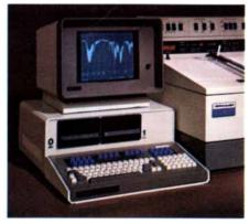
Perkin-Elmer IR Data Station can overlay two spectra and highlight differences between them (bright band on screen).
