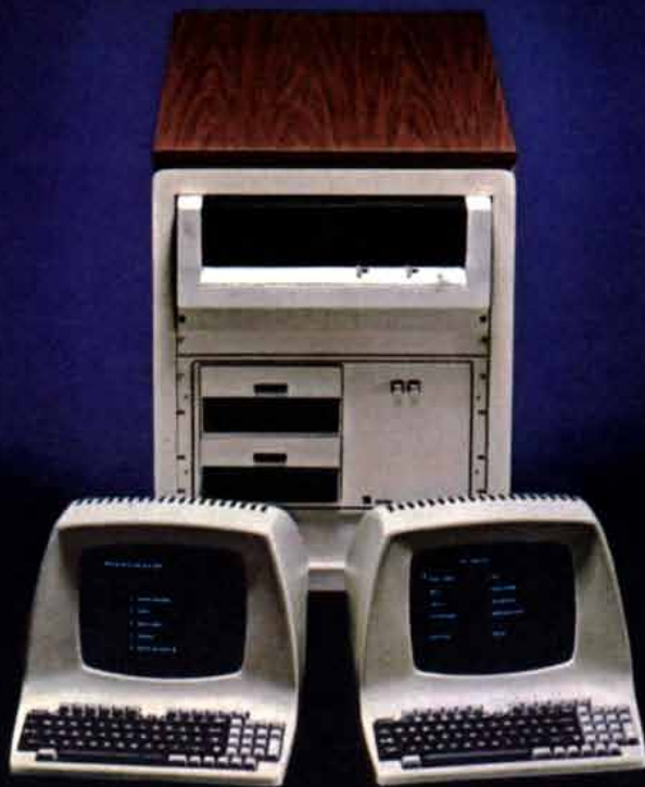
Zilog MCZ-1/70 microcomputers can support five terminals, giving multiple users access to the same information.
