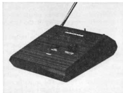
The base unit for the Mura can also be used as a personal paging system or intercom.
