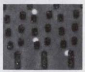
In this photo, magnetic bubbles (white dots) are magnified 1,000 times.
