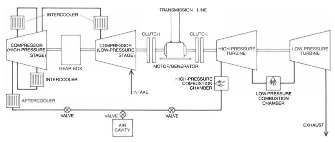
COMPRESSED-AIR ENERGY-STORAGE PLANT, the first of its kind, is now operating at Huntorf, near Bremen in West Germany. In periods of low demand (typically over an eight-hour night period) air is compressed and stored at a pressure of about 70 atmospheres in two caverns leached out of a salt dome that have a combined capacity
