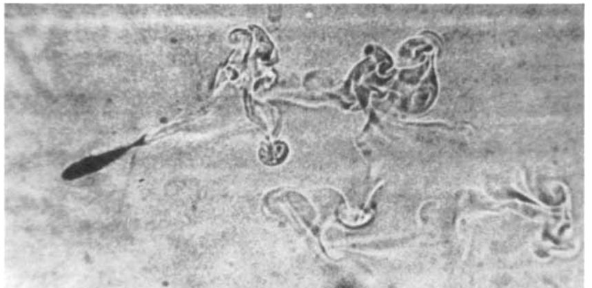
A shadowgraph of a small fish swimming in the "push and coast" mode
