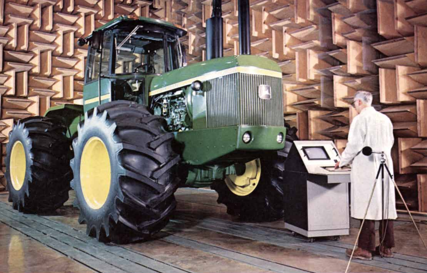
This technician is taking a sound signature to identify and isolate noise sources. Deere controls noise while developing machines that operate with increased power and speed.
