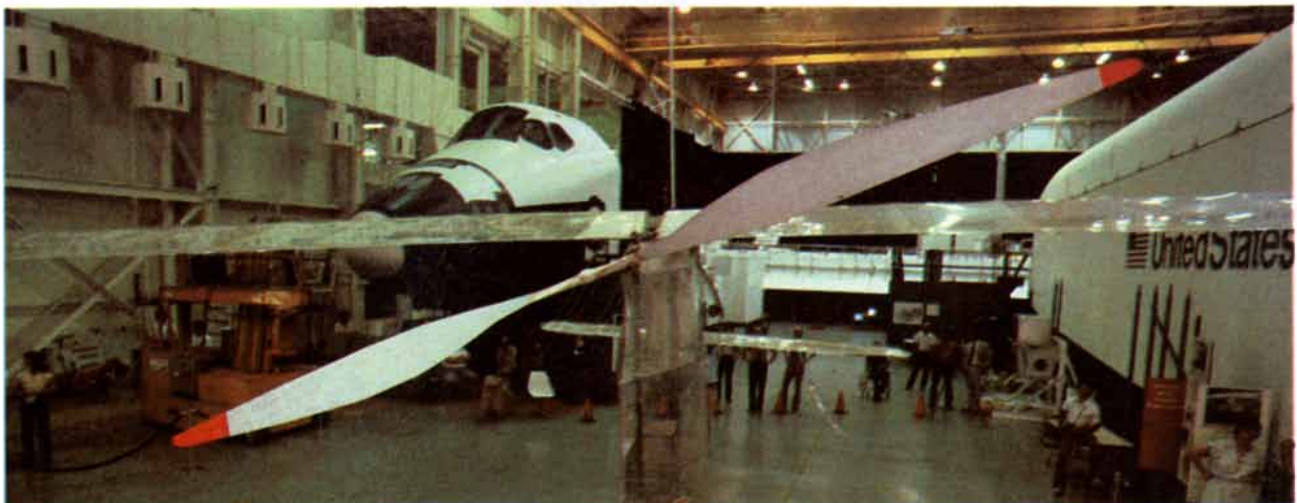
PROPELLER OF "GOSSAMER ALBATROSS," the ultralight aircraft Bryan Allen pedaled across the English Channel on June 12, 1979, bears only a remote resemblance to the screw of Queen Elizabeth 2 shown at the top of the page. Both propellers, however, act as "pushers" and are among the most efficient of their type ever designed. The airscrew of the Gossamer Albatross is 4.1 meters in diameter,
