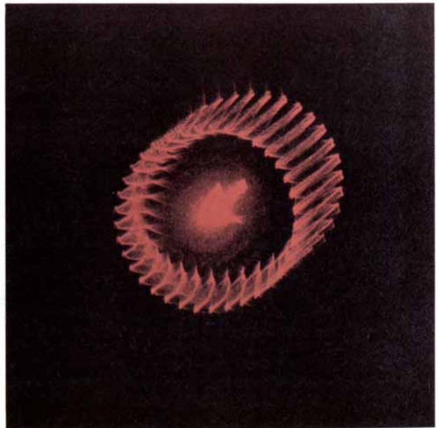
A 48-segment grating combined with textured plastic
