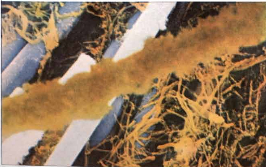
Color-enhanced scanning electron micrograph showing the results of lithium attack on boron nitride.
