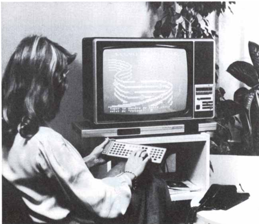
This home terminal was developed by Thomson-CSF Telephone for the French videotex network which becomes operational in the Paris suburb of Vélizy later this year. It is connected directly through the telephone network to information stored in data bases.
