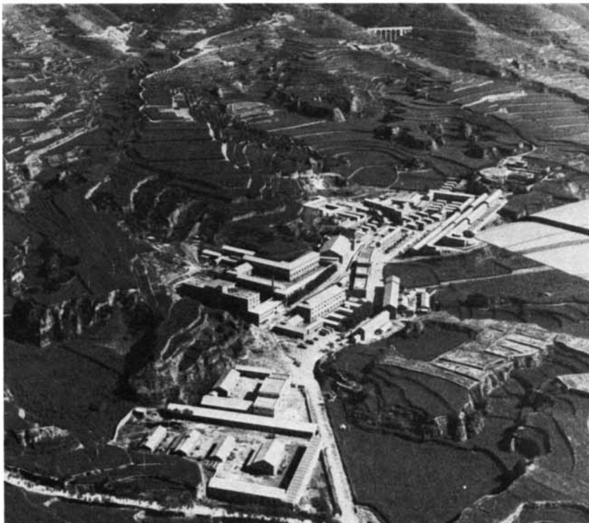
TERRACED FIELDS of Dazhai, once a small village in the barren hills of Shanxi Province, are one of China's showplaces. In the 1940's the 60 hectares of arid farmland here were split into nearly 5,000 separate parcels occupying eight ridges and seven gullies. Villagers have now terraced the hillside fields, filled in four of the gullies and constructed an irrigation system.
