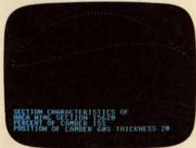
Apple's existing software library includes a program that plots the shape of an airfoil, given its parameters.
