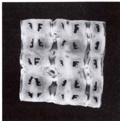
MATRIX MIRROR consists of four or more basic regions joined by bell boundaries. In this example, convex, concave and saddle-shaped regions are brought together in a repeated two-by-two pattern. Because there are bell boundaries on at least two sides of each basic region, it is possible to generate as many as four images in each two-by-two cell of the matrix. By tilting the mirror obliquely double pairs of enantiomorphic images can be annihilated and created.
