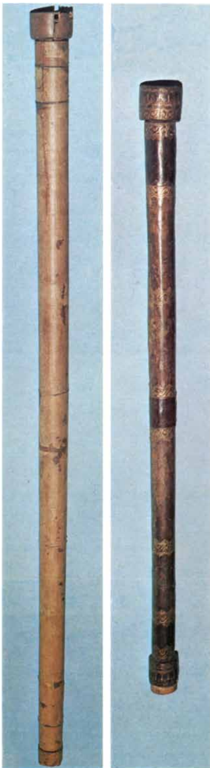
TWO TELESCOPES thought to have been made by Galileo are preserved at the Institute and Museum for the History of Science in Florence. The instrument at the left has a magnification of 14, a resolving power of 20 arc seconds and a field of view of 17 arc minutes. Instrument at the right has a magnification of 20, a resolving power of 10 arc seconds and a field of view of 17 arc minutes. The actual telescope employed by Galileo in his observations of Neptune (which has not been preserved) had a magnification of 18 and a resolving power of 10 arc seconds; the field of view was probably 17 arc minutes.
