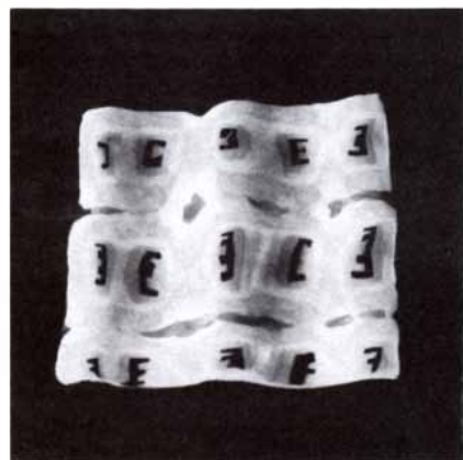
MATRIX MIRROR consists of four or more basic regions joined by bell boundaries. In this example, convex, concave and saddle-shaped regions are brought together in a repeated two-by-two pattern. Because there are bell boundaries on at least two sides of each basic region, it is possible to generate as many as four images in each two-by-two cell of the matrix. By tilting the mirror obliquely double pairs of enantiomorphic images can be annihilated and created.
