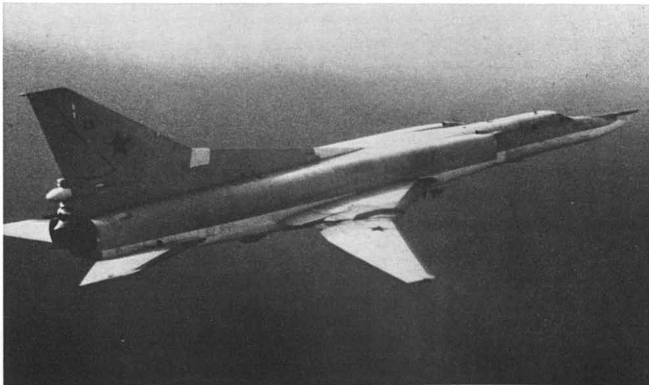
NEW RUSSIAN BOMBER , the medium-range, swept-wing Tu-26 (also known in the West as the Backfire), is seen in a photograph supplied by the Swedish Air Force. The probe projecting from the nose is for in-flight refueling, which some Western analysts believe gives the bomber a strategic, or intercontinental, capability. Without
